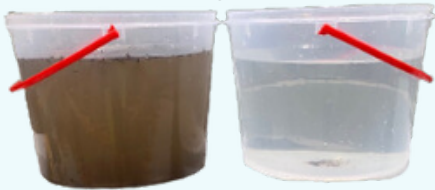
(Left) Natural Stormwater (Right) Results after single pass in Enviro H45
