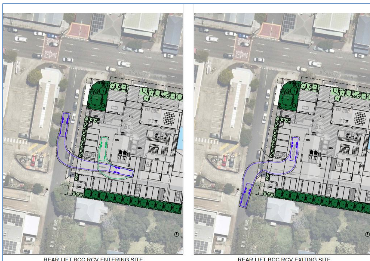
Figure 2.2 illustrates the swept paths for the rear loading RCV. Further details on vehicle access and on-site manoeuvring can be found in the transport report submitted with the submission.
