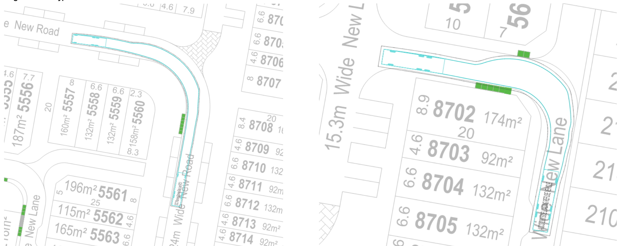
Figure 4-4.1: Typical Bin Pad Locations
