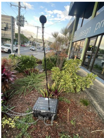
Figure 2 Noise logger at the noise monitoring location
