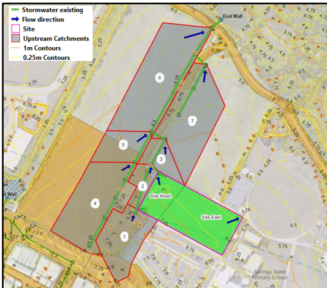
Figure 5.1: Overview of existing stormwater infrastructure and catchments
