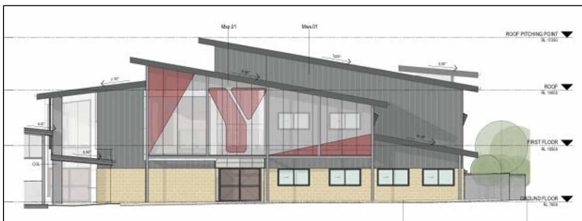
Figure 12: North-west elevation of school buildings (seen from internal car parking area) showing varied roof forms and overall height of 2-3 storeys
