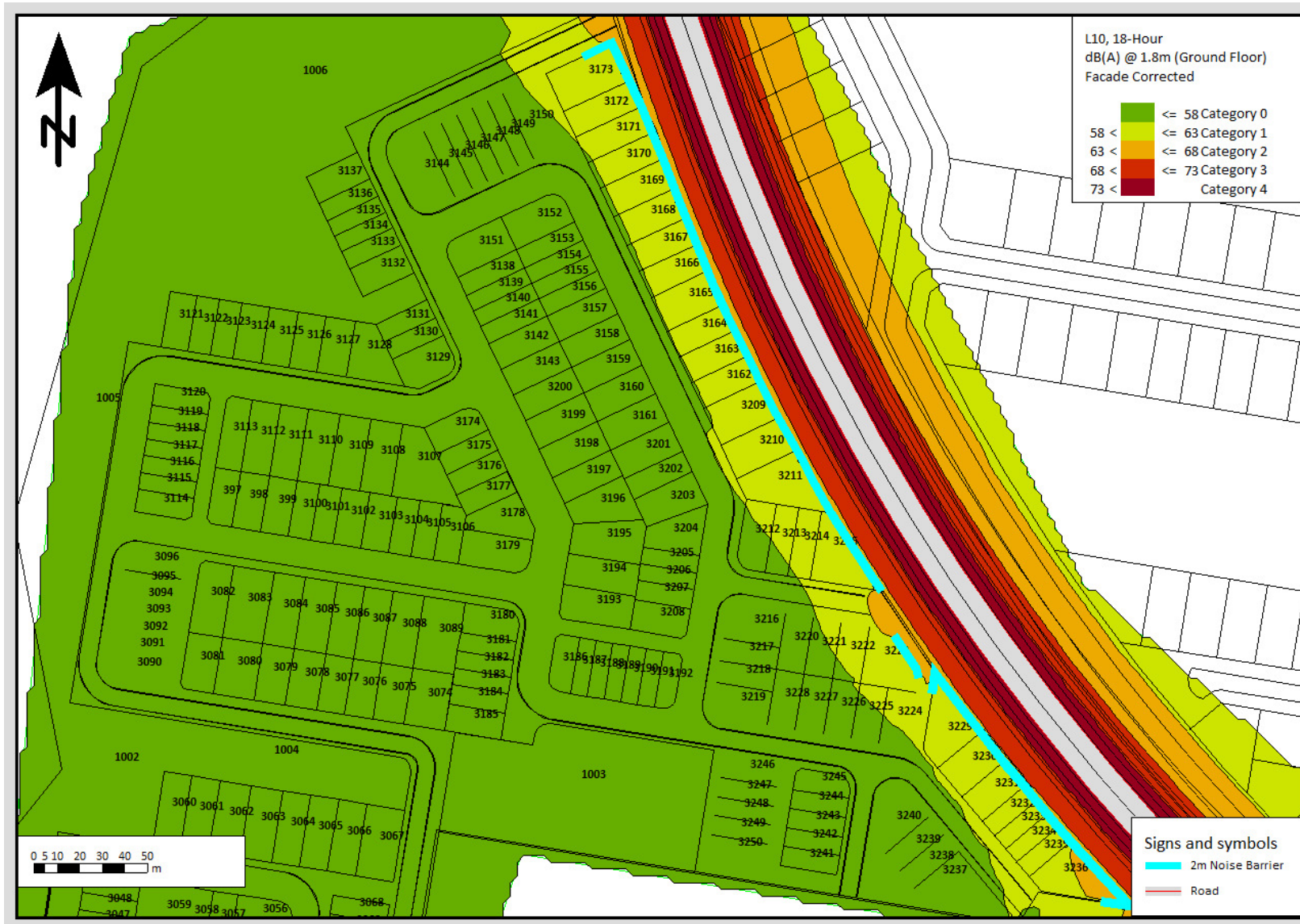
Figure A-1: Ground Floor Noise Contour Map with QDC MP4.4 Categories (Façade Corrected)
