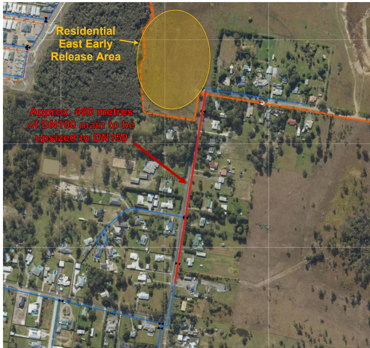
Figure 4-7: Option 2 – Upsize the DN100 main coloured in red on Farry Road to a DN150 main
