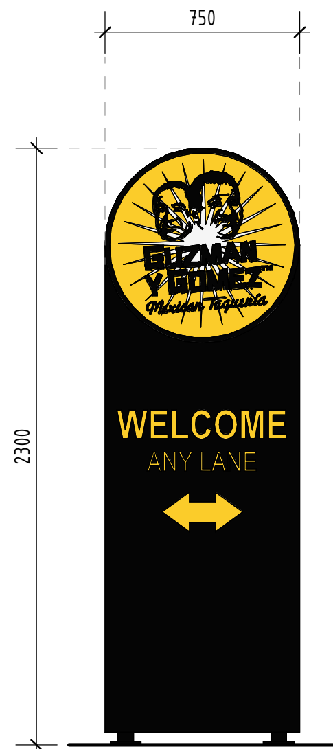
2 D-01 - ILLUMINATED DIRECTIONAL SIGNAGE - 1 OFF 1 : 20
