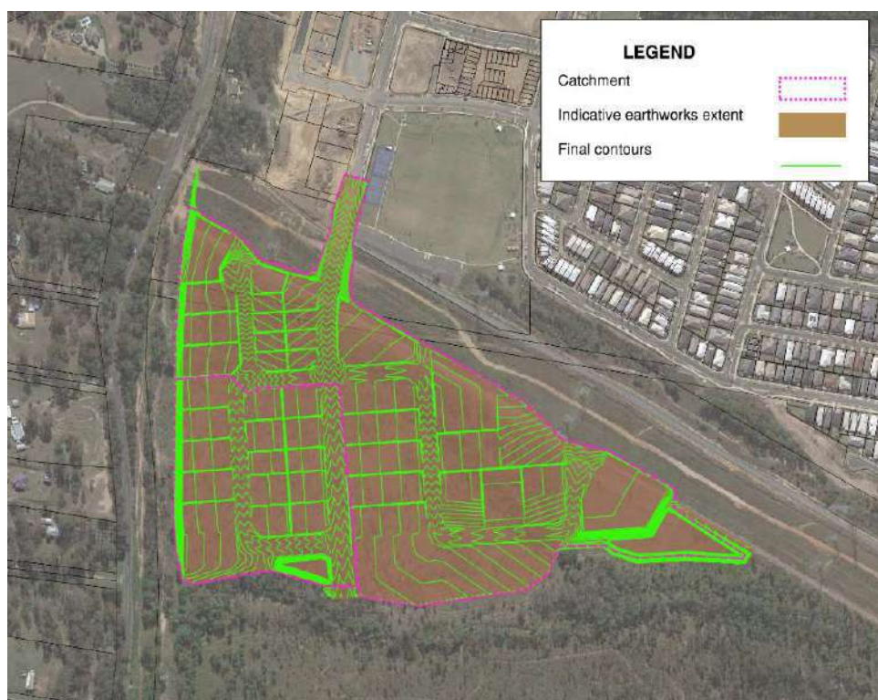
Figure 2: Bulk earthworks extent
