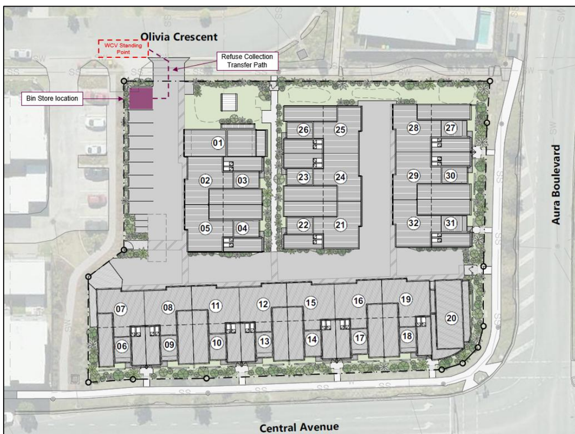
Figure 2 – Refuse Collection Transfer Path
