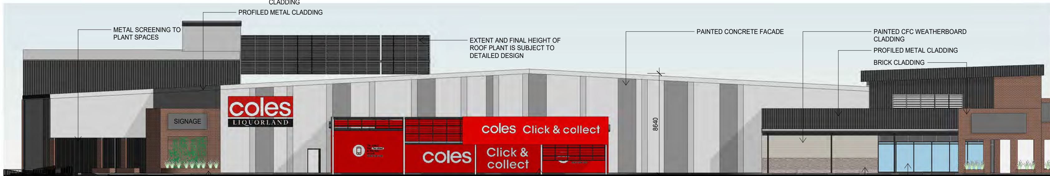
3 BUILDING 1 - SOUTH ELEVATION 1: 200
