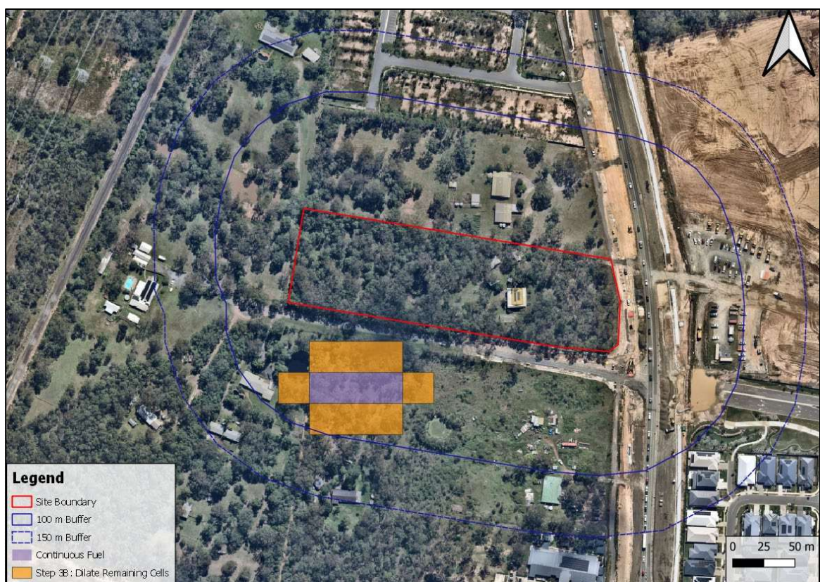
Figure 10. Step 3b – Dilation of residual continuous fuel patches
