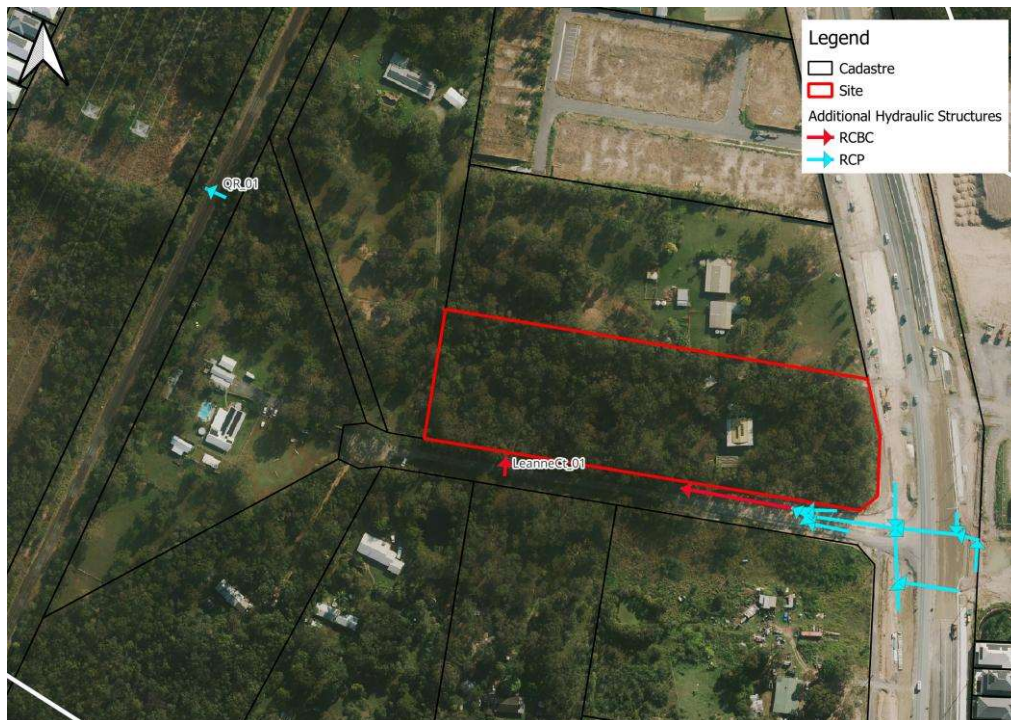
Figure 5-2 Key Hydraulic Structures – Existing Conditions
