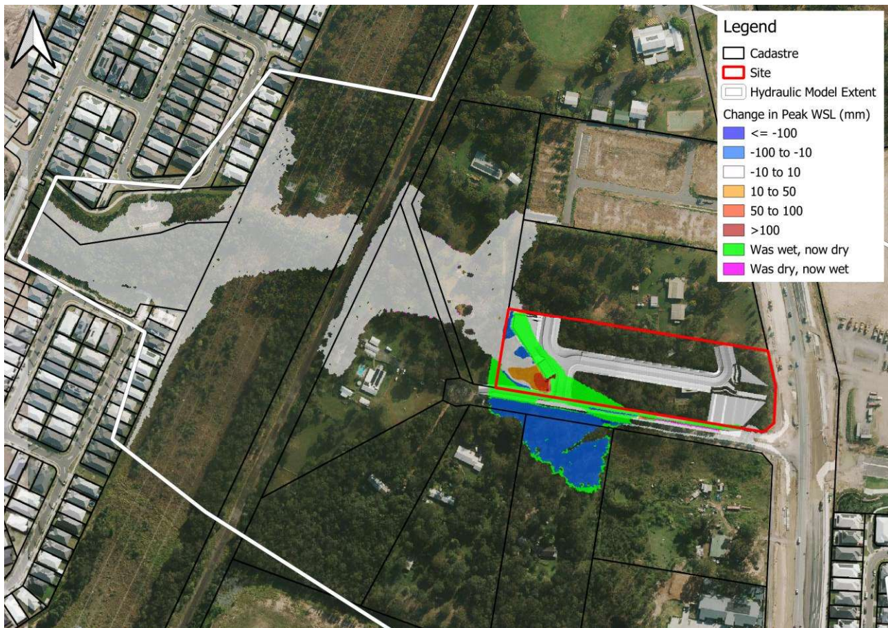
Figure 5-6 1% AEP Design Event Afflux Results
