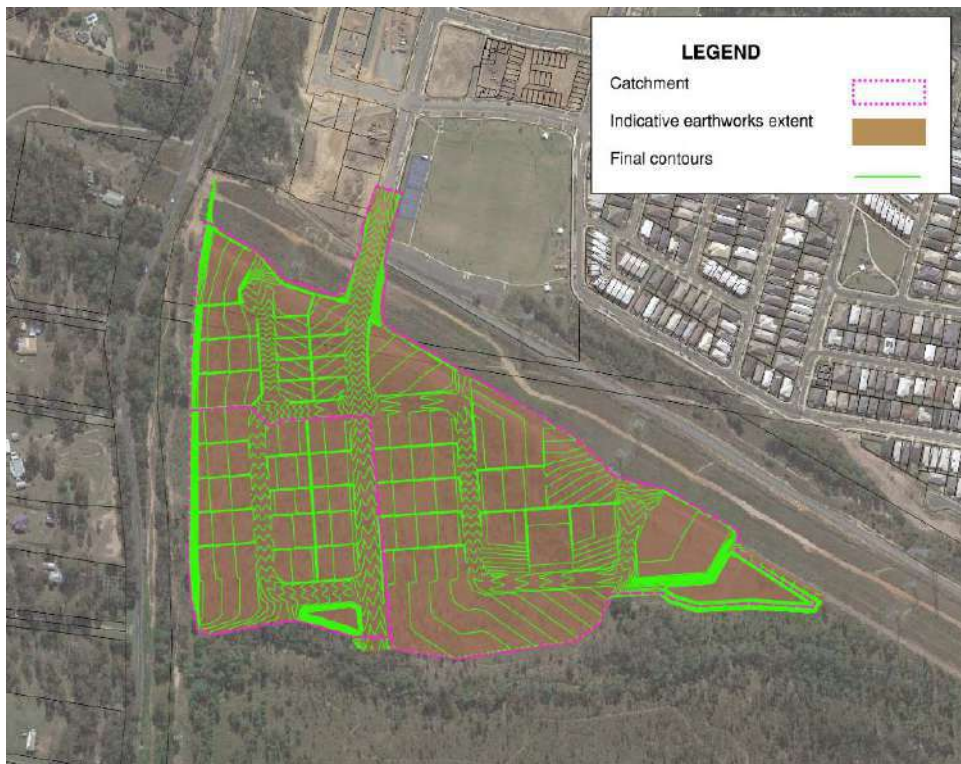
Figure 2: Bulk earthworks extent
