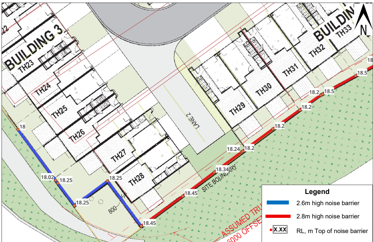
Figure 4.2 Noise barrier alignment – Part 1
