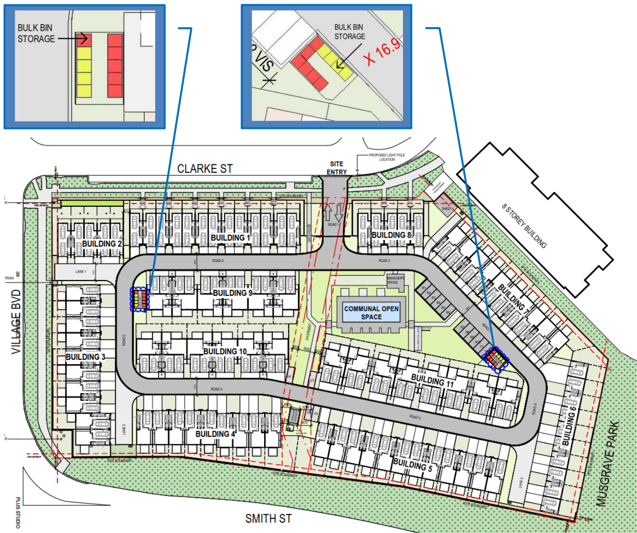
Figure 2.3: Residential Refuse Storage Room
