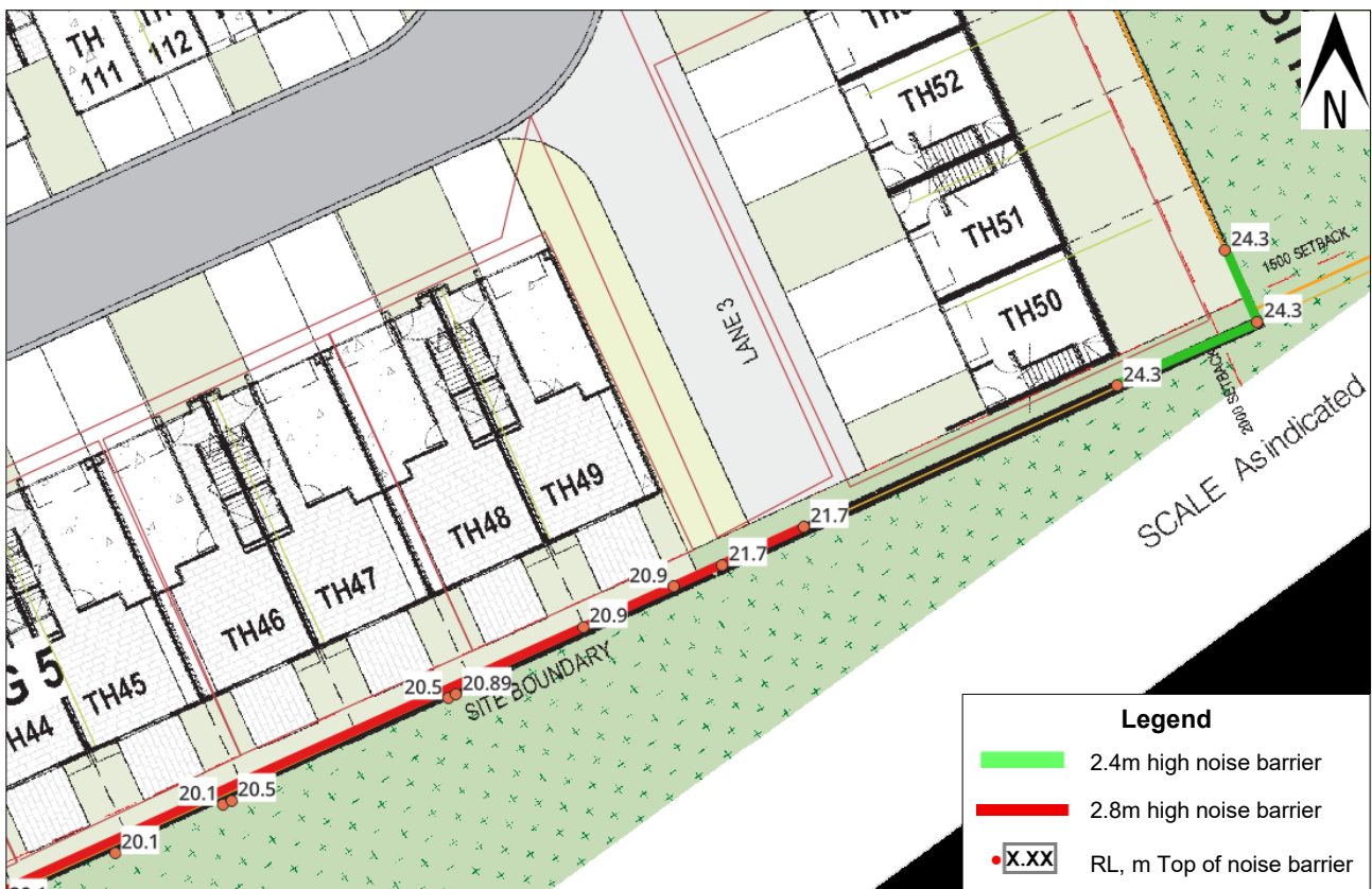
Figure 4.4 Noise barrier alignment – Part 3
