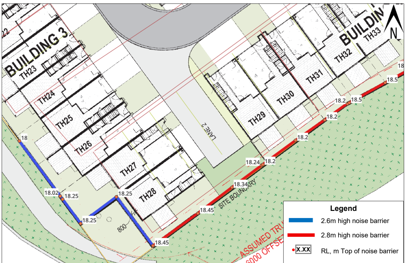
Figure 4.2 Noise barrier alignment – Part 1
