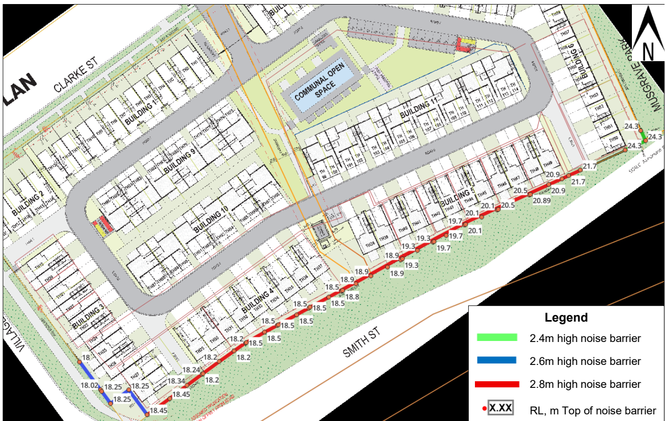
Figure 4.1 Noise barrier alignment – Total
