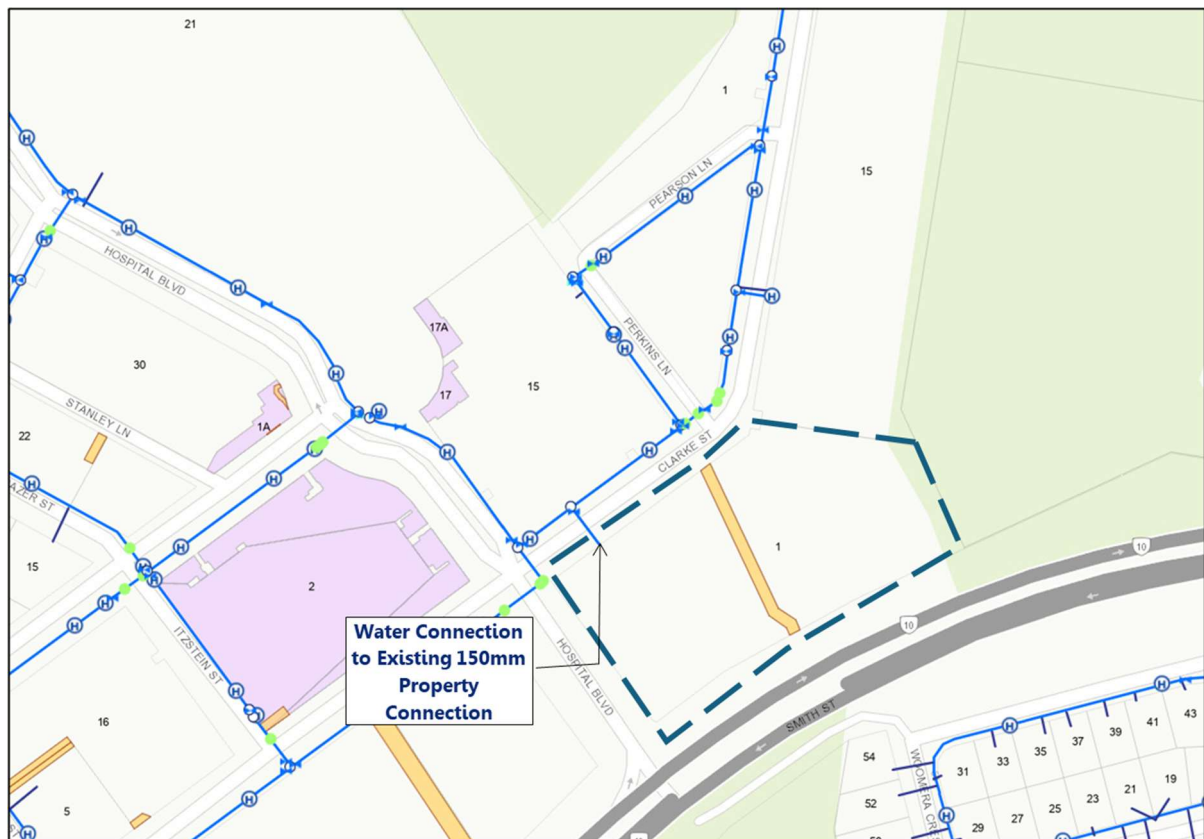
Figure 7.1 – Existing Water Infrastructure & Proposed Connection Location
