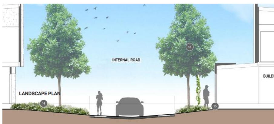
Figure 15: Section – Internal loop road with pedestrian-priority pathways
