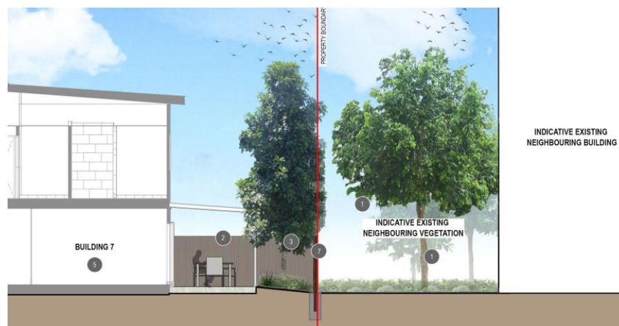
Figure 35: Smith 19 Section – Building separation and landscape features
