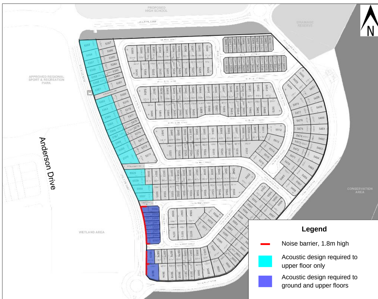
Figure 6.1 Noise control measures – RoL 21
