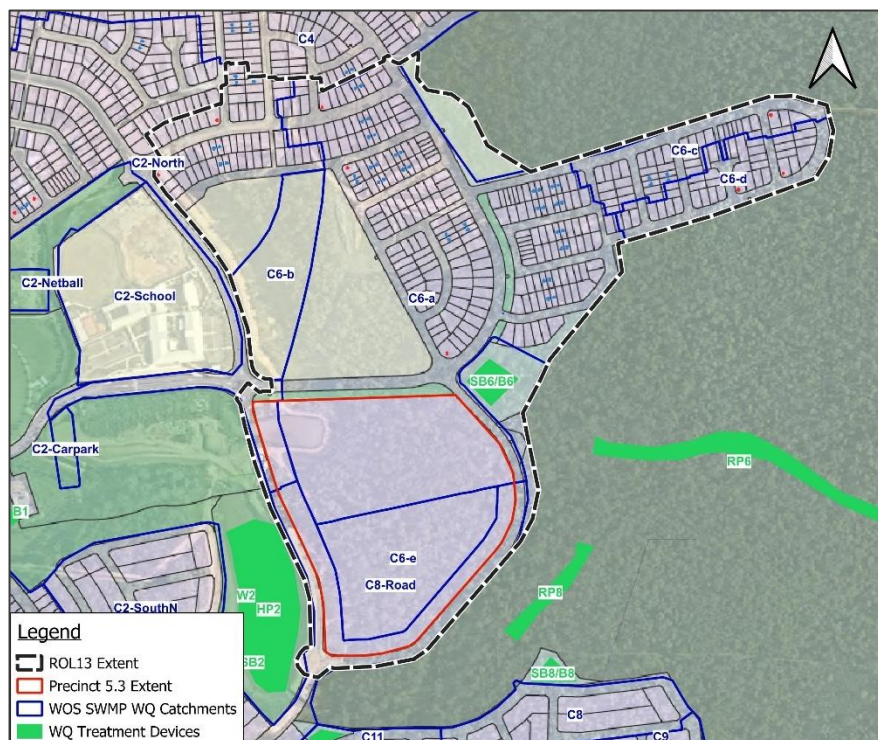
Figure 3: Precinct 5.3 Stormwater Quality Catchments
