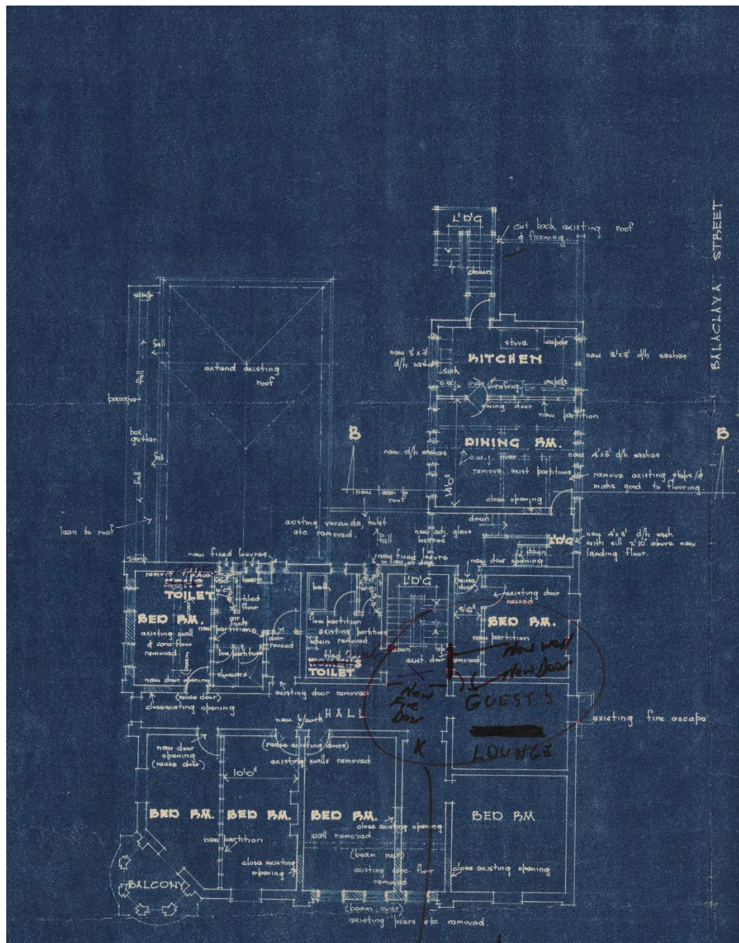
Figure 7 First floor plan showing 1958 alterations and additions Source: QSA
