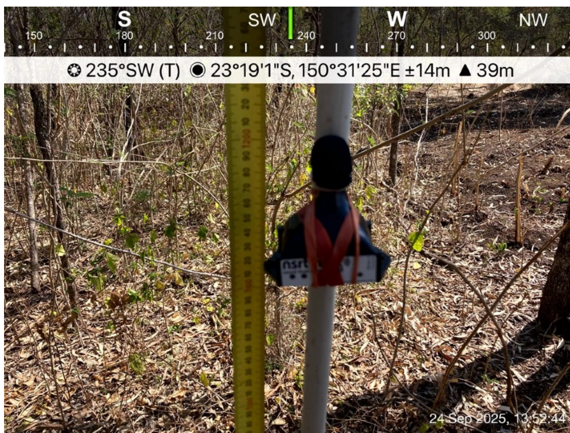
Figure 4, Sound logger in situ
