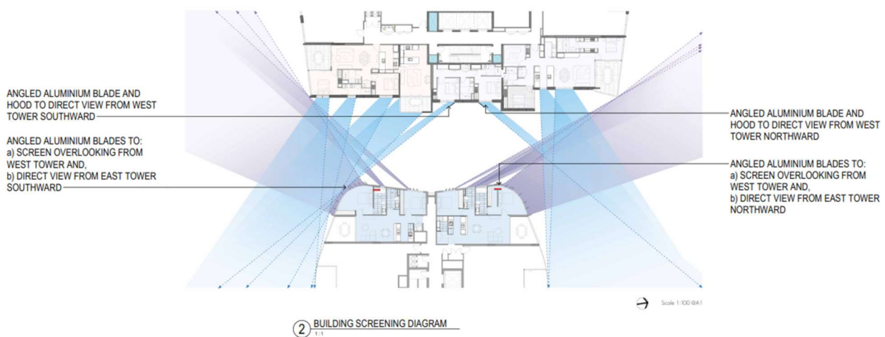
Figure 12: Context plan showing unit interface and orientation between East and West towers (GroupGSA)
