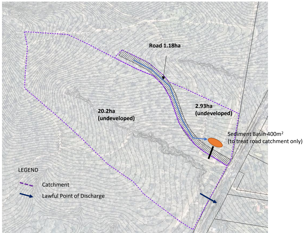
Figure 3 Interim stormwater treatment strategy
