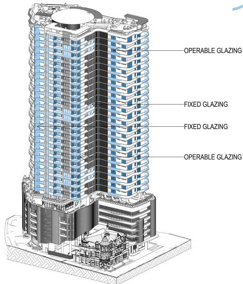
NATURAL VENTILATION DESIGN - 3D VIEW
