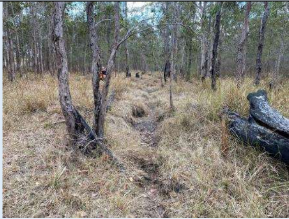
CH820-950 Minor low flow channel (periodically) but very localised and on very low gradient. Scattered shallow scour pools (dry) likely partly from livestock trail and disturbance. Low risk. Monitor and plant disturbed areas if natural regeneration is slow.
