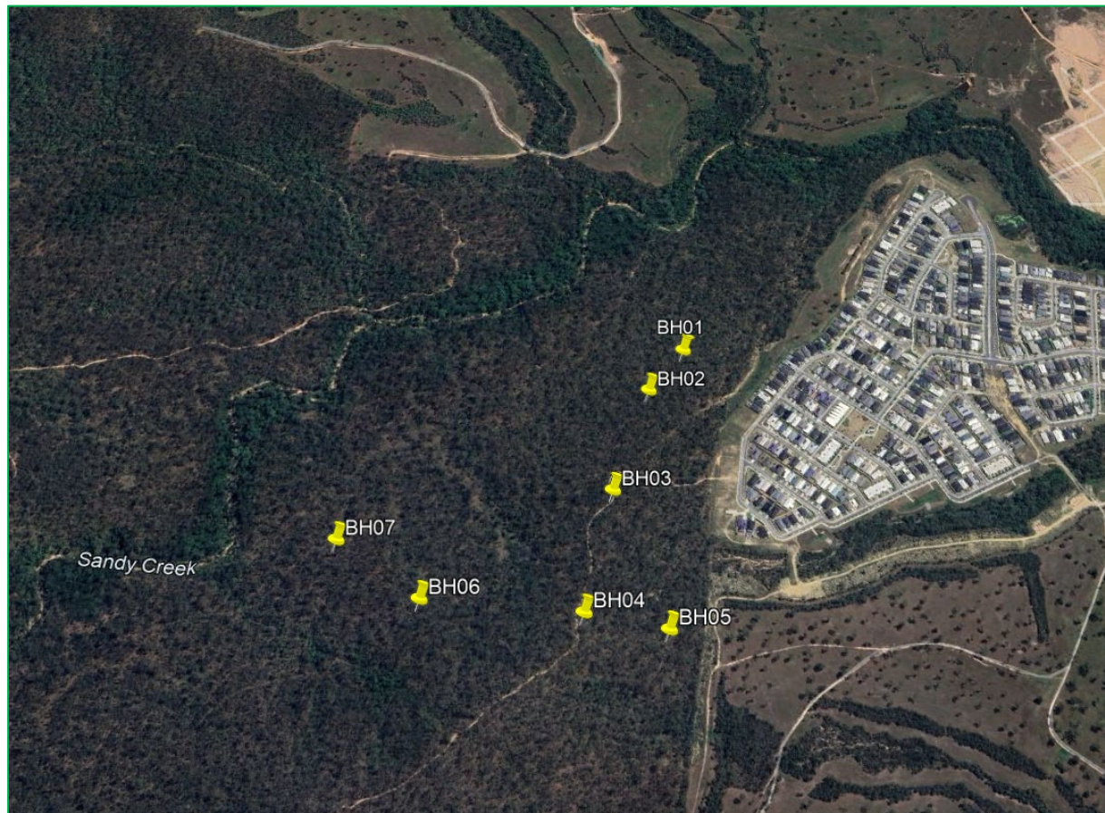
Figure 5: Site Plans Showing Test Locations
