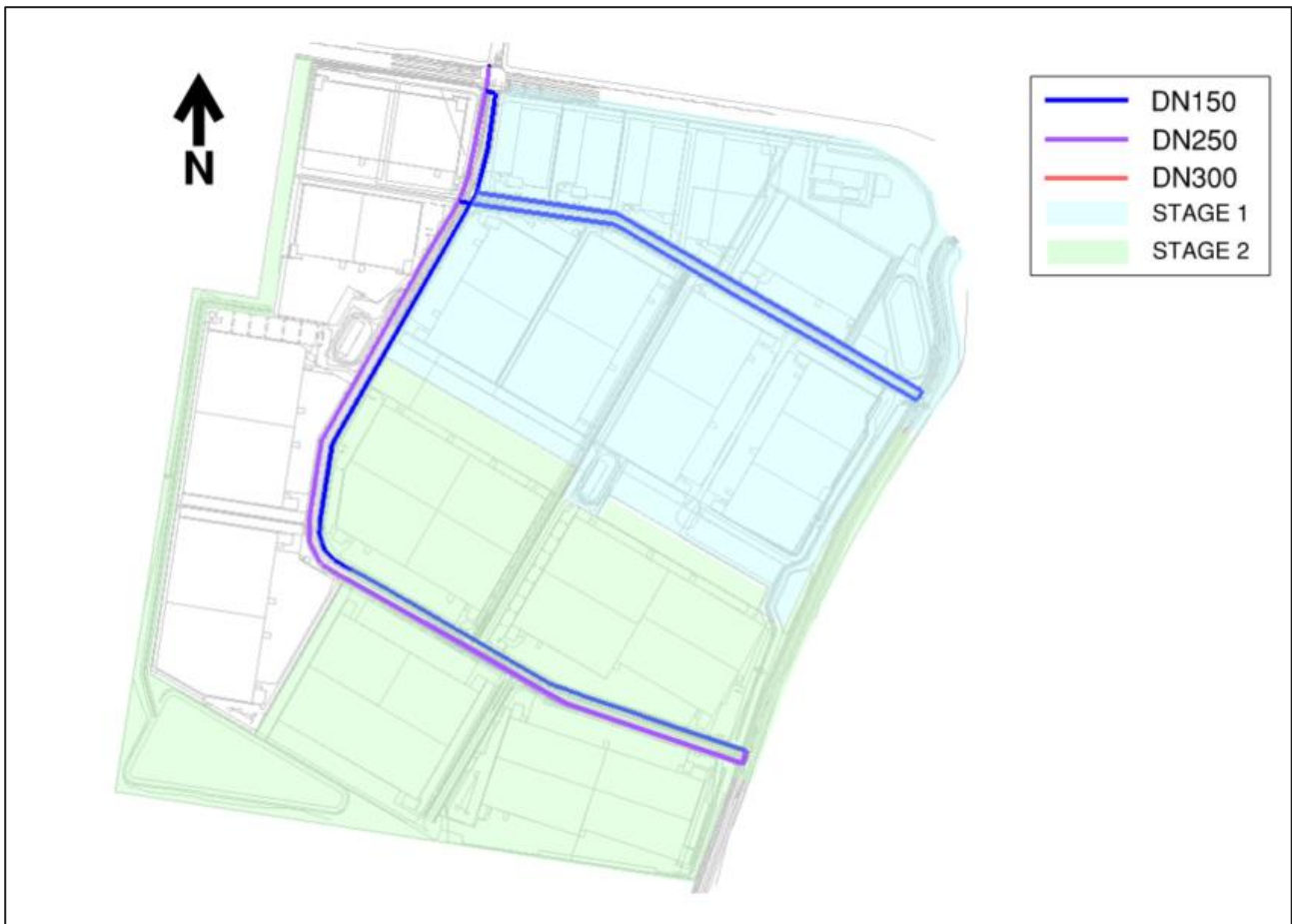
Figure 9-3 Concept Stage 1-2 Internal Water Network Layout
