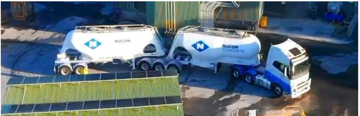
Figure 2. Typical tanker used for the delivery of cementitious materials.
