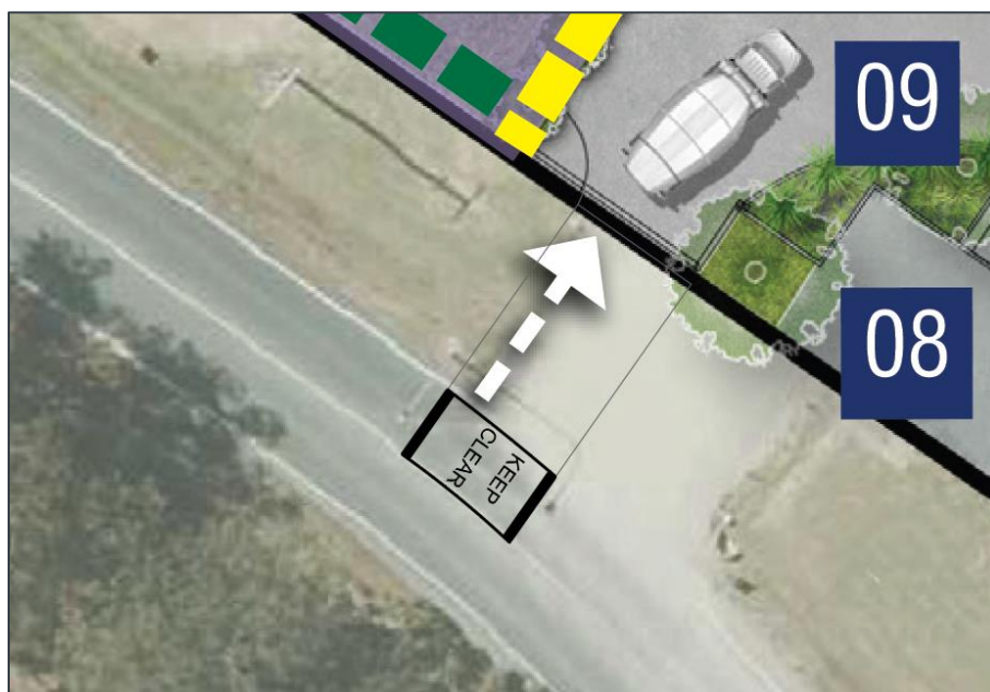
Figure 9.2 Concept Design – Keep Clear Pavement Markings
