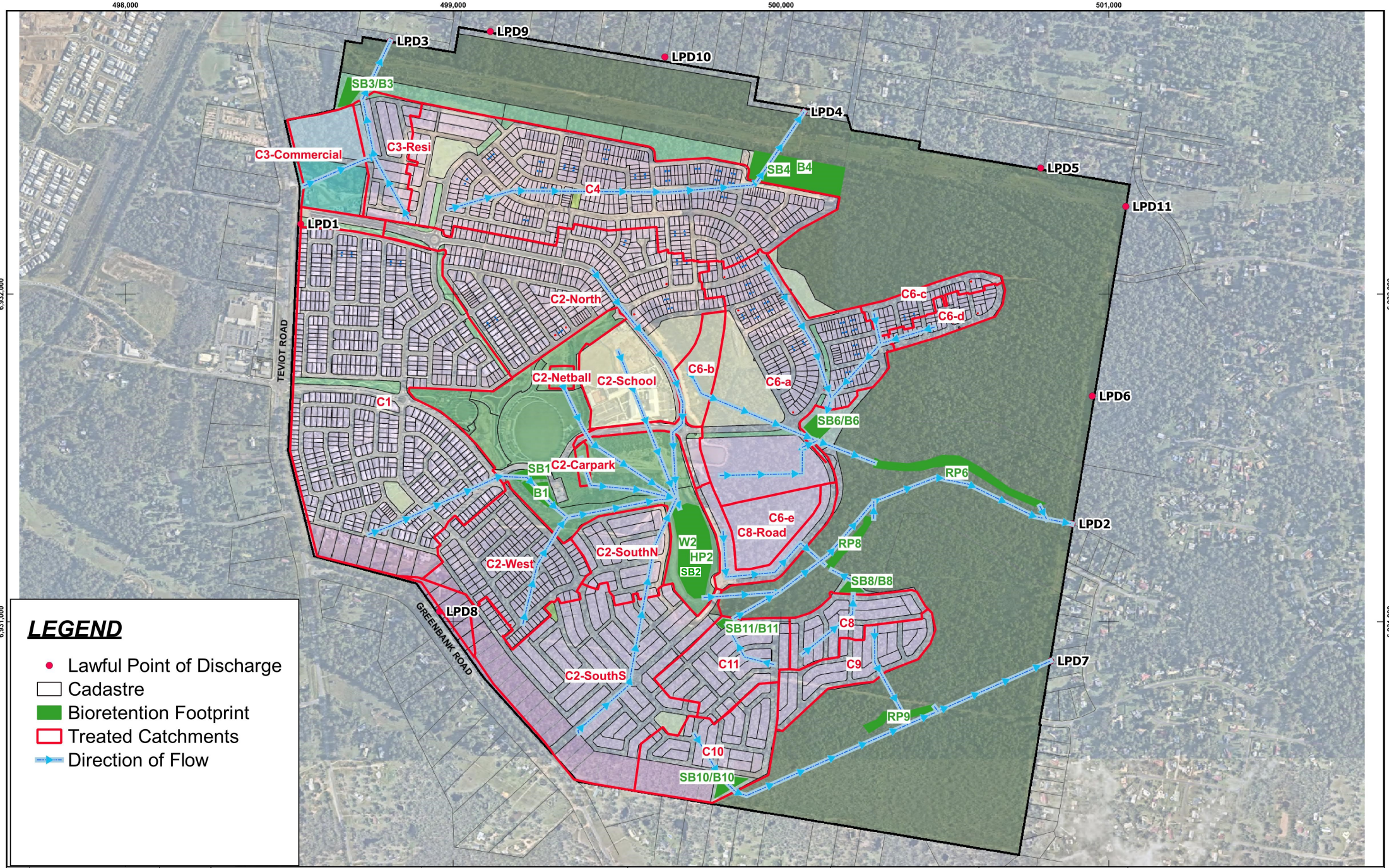
Figure F3 Mirvac Everleigh Masterplan Update Stormwater Treatment Locations and Contributing Catchments Dwg Ref: QC4060-005-SKE-0002
