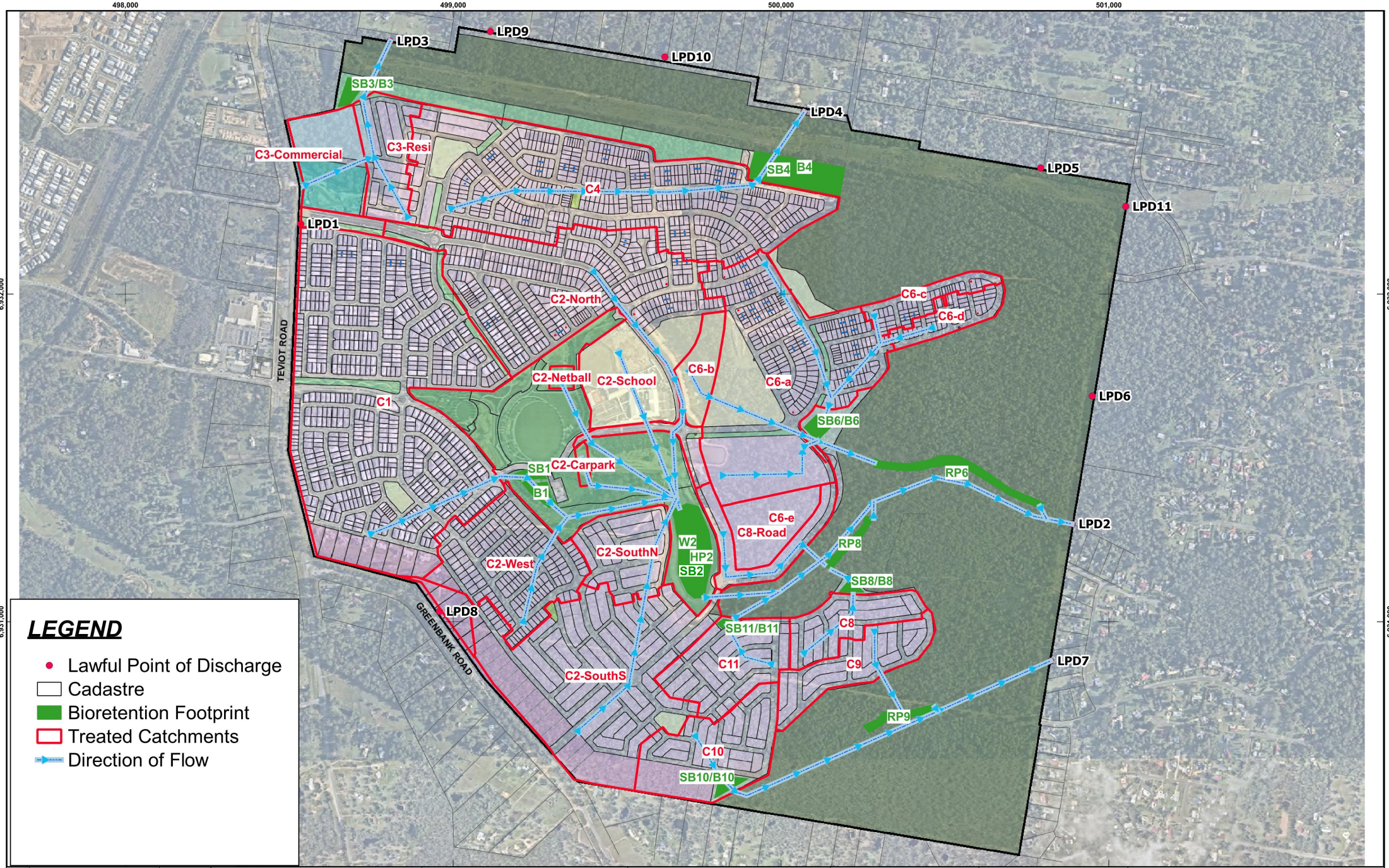
Figure 4.2 Mirvac Everleigh Masterplan Update Stormwater Treatment Locations and Contributing Catchments Dwg Ref: QC4060-005-SKE-0002
