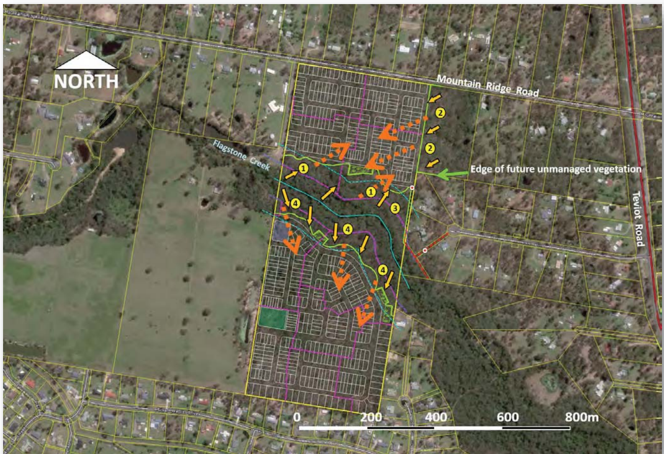
Figure 4. Fuel Zones Assessed Solid orange arrows indicate most likely direction of bushfire attack, dotted arrows in the form of embers. Contours shown are 5m.
