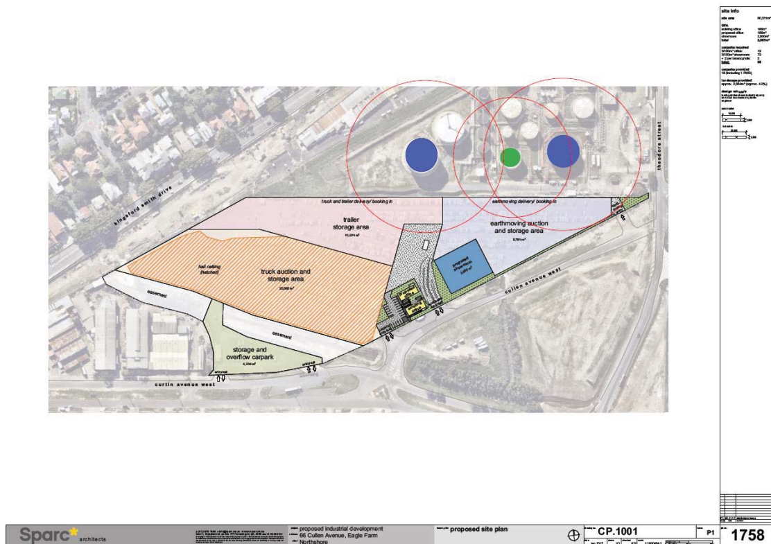
Figure 4: 4.7 kW/m 2 Heat Flux contours for Petrol and Diesel Fires.
