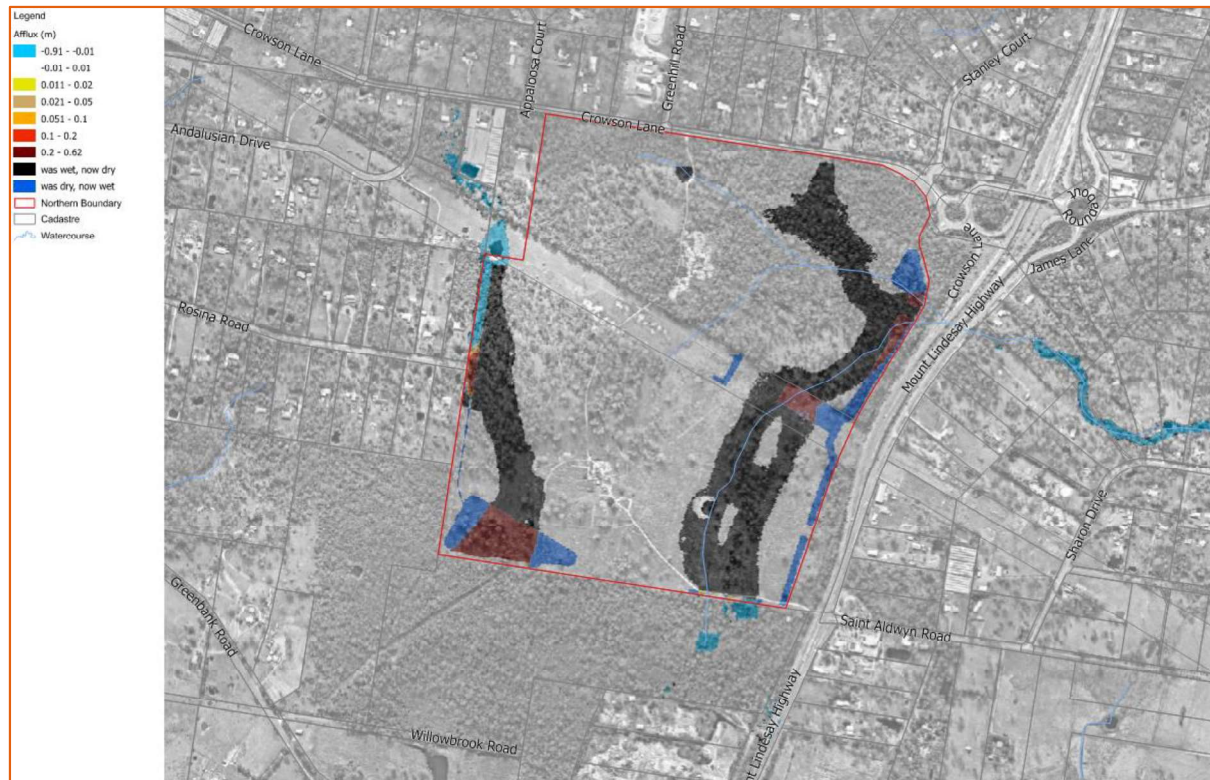
Figure 6-5 - Developed Peak Water Surface Level Change - 1% AEP
