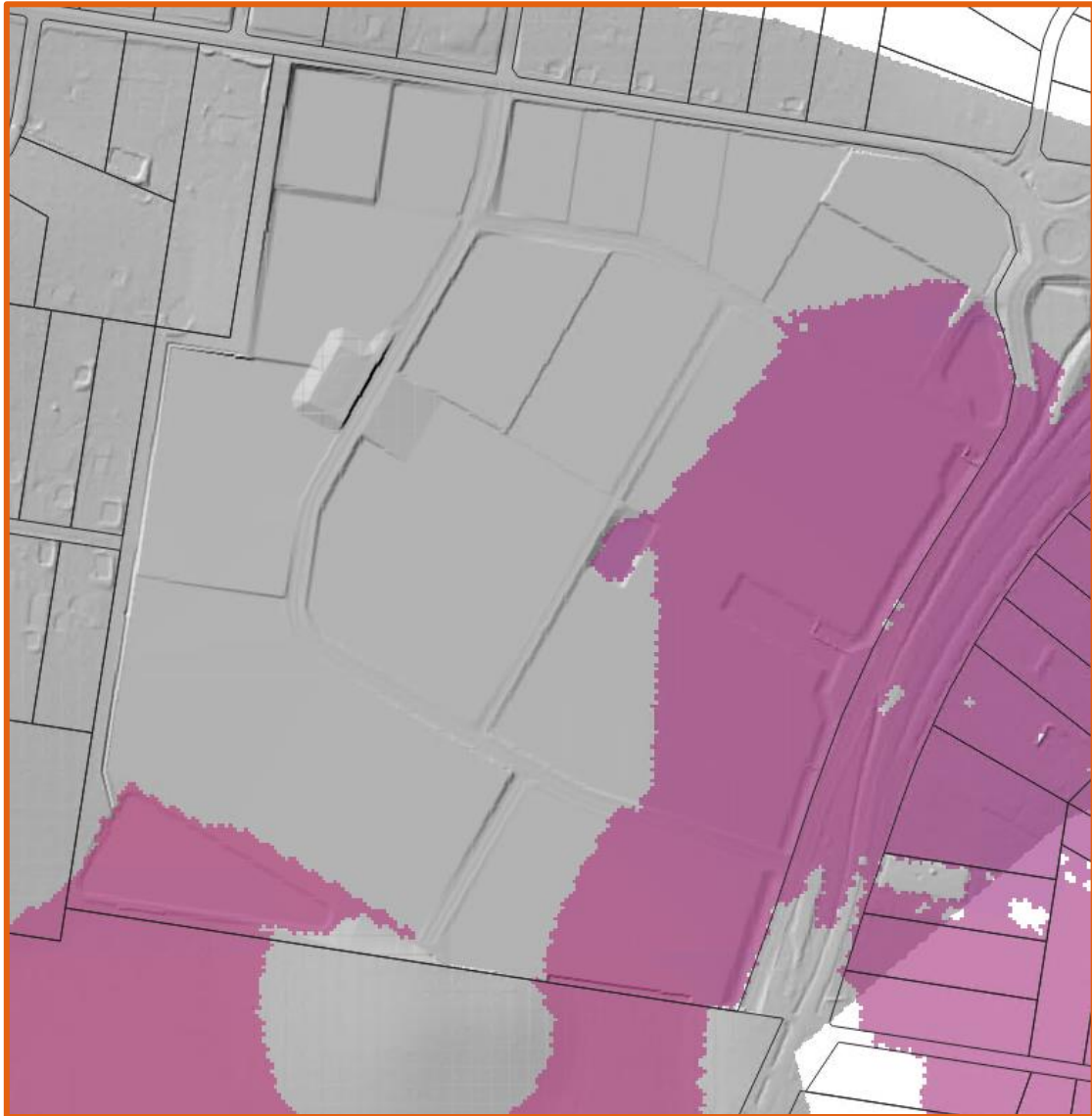
Figure 7 – Base Case 0.2% AEP (500 year) at 2100 flood inundation.
