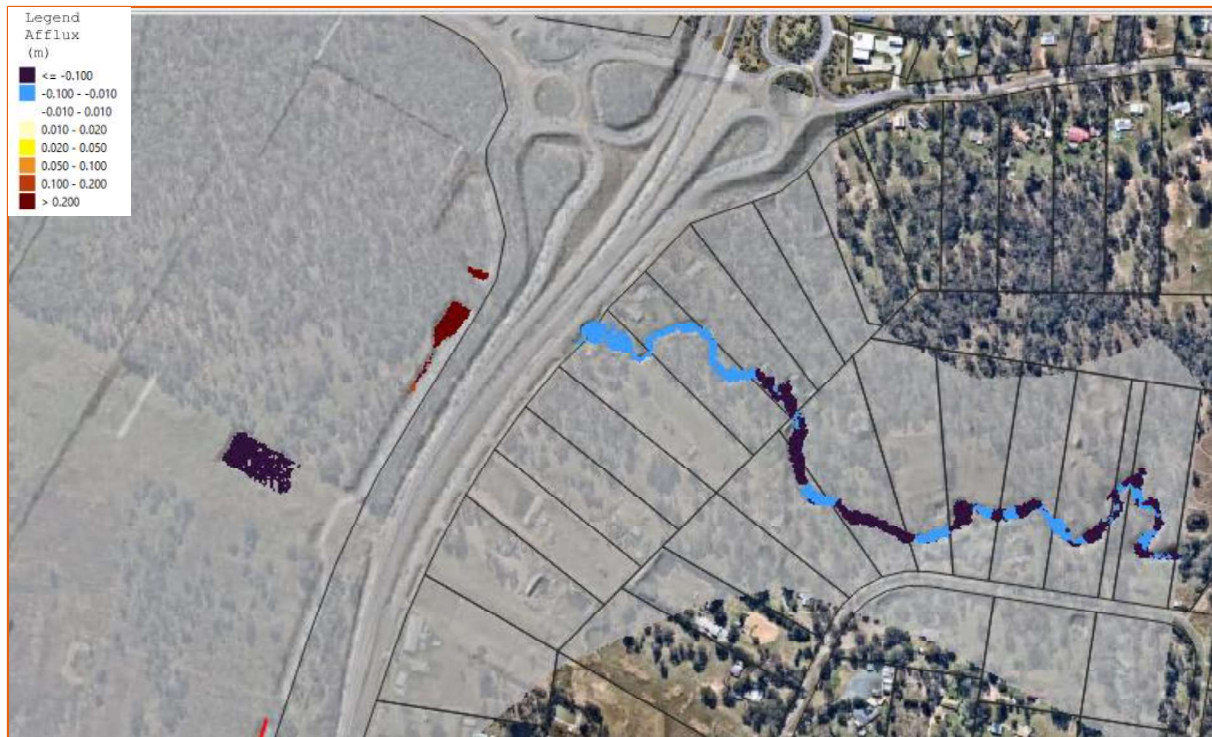
Figure 6-13 - Developed Peak Water Surface Level Change - 50% AEP
