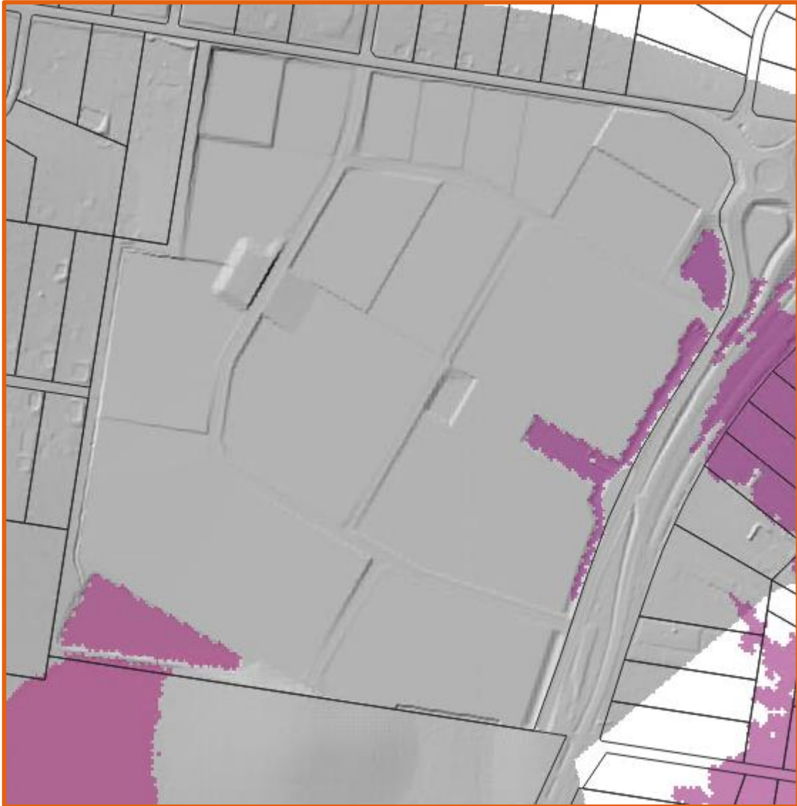
Figure 6 – Base Case 1.0% AEP (100 year) at 2100 flood inundation.
