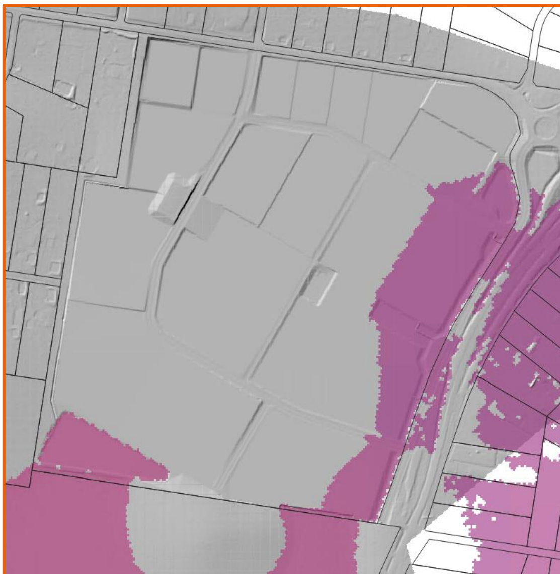
Figure 8 – Base Case 0.5% AEP (200 year) at 2100 flood inundation.
