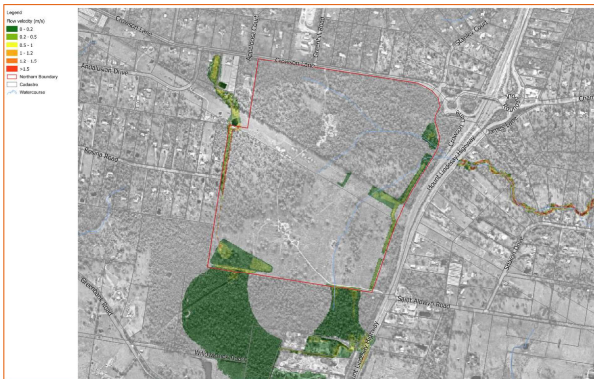
Figure 6-7 - Developed Peak Water Velocity - 1% AEP
