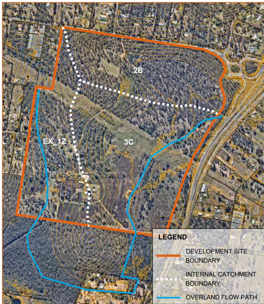
Figure 3-2- Internal Catchment Plan (Source: NearMap, June 2022)
