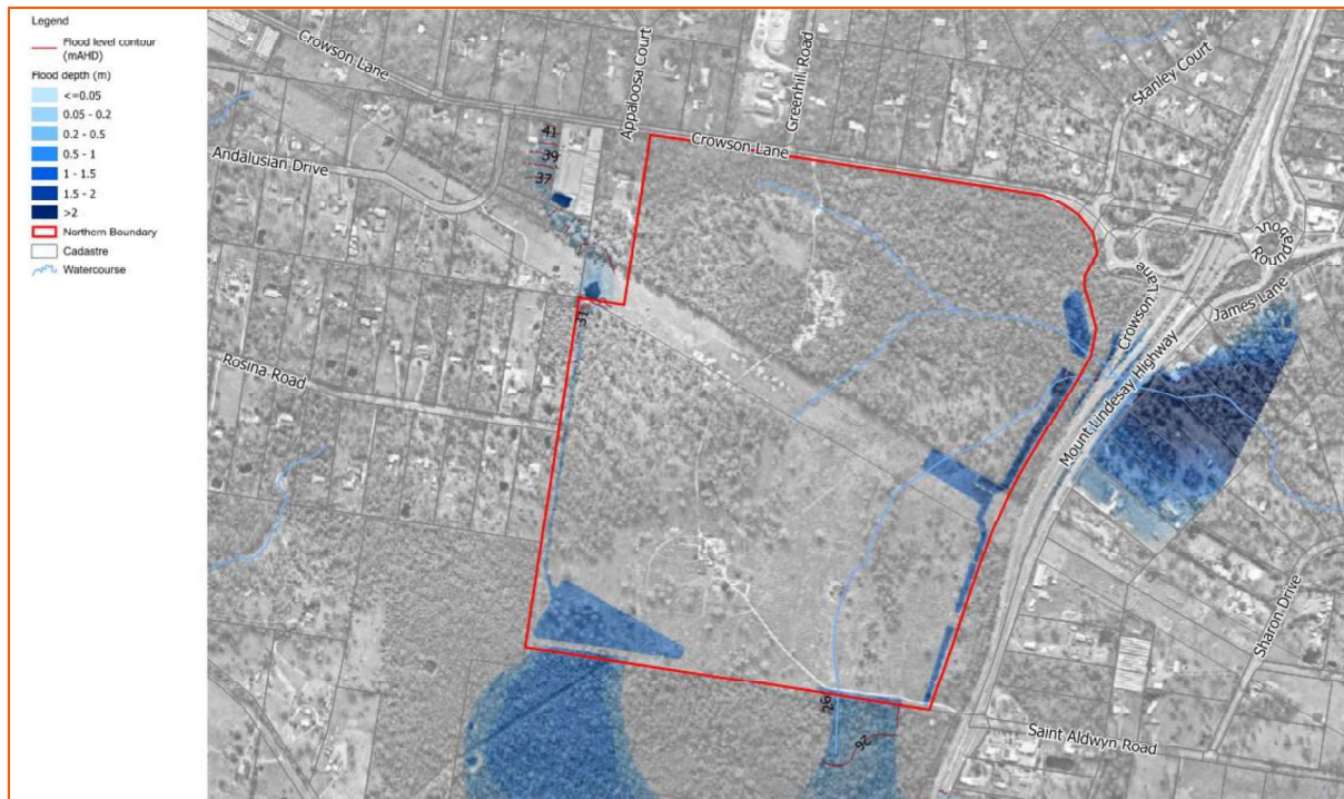
Figure 6-10 - 1% AEP 72hr Regional Flood Depth and Extents
