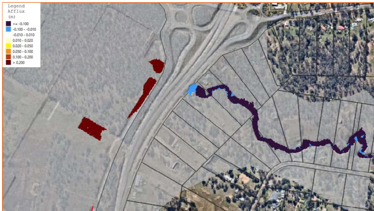
Figure 6-14 - Developed Peak Water Surface Level Change - 1% AEP
