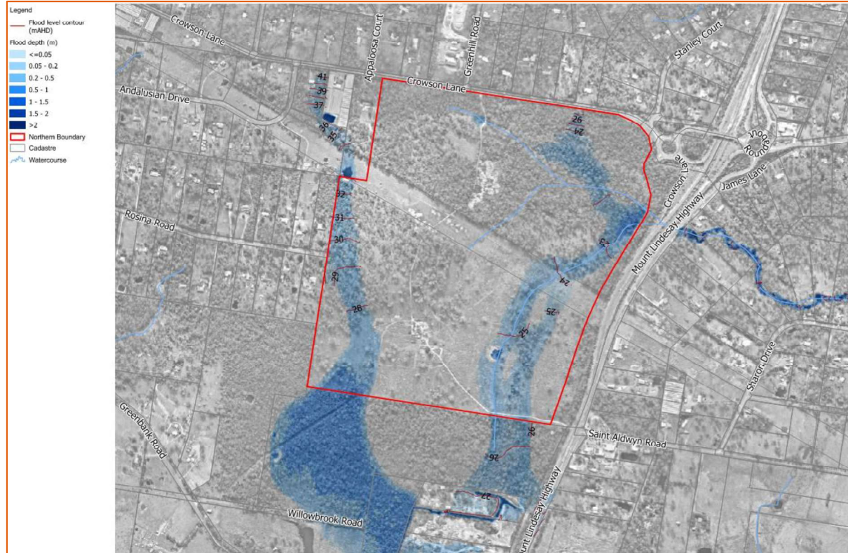
Figure 6-1 - Existing Peak Water Depth - 1% AEP
