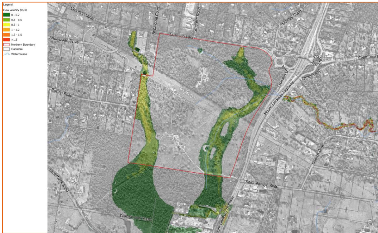
Figure 6-6 - Existing Peak Water Velocity - 1% AEP
