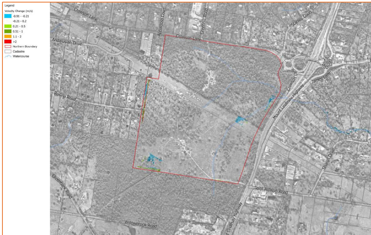
Figure 6-8 – Change in Flow Velocity - 1% AEP
