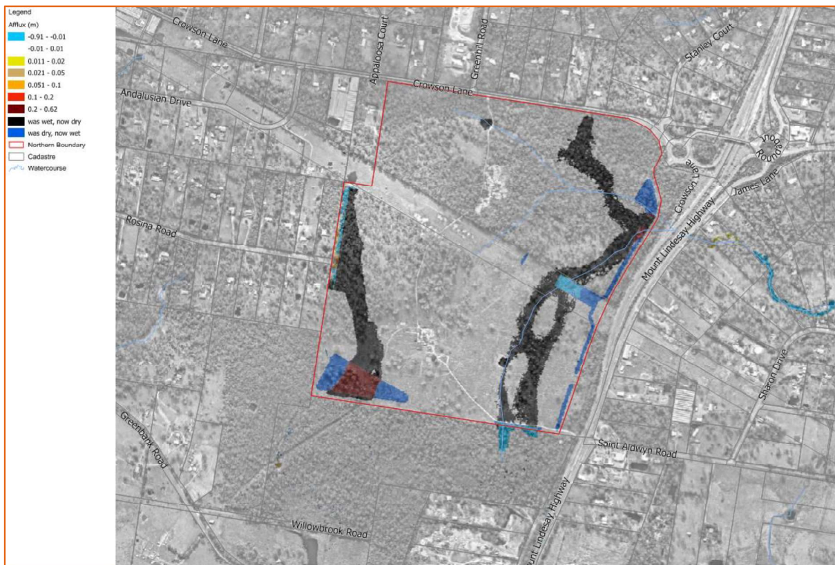
Figure 6-4 - Developed Peak Water Surface Level Change - 50% AEP
