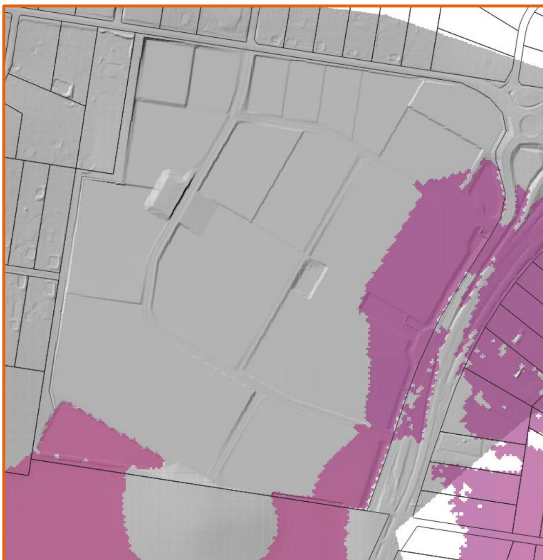
Figure 8 – Base Case 0.5% AEP (200 year) at 2100 flood inundation.
