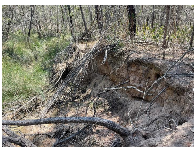
Location 4 – Scour and Dispersive Soils
