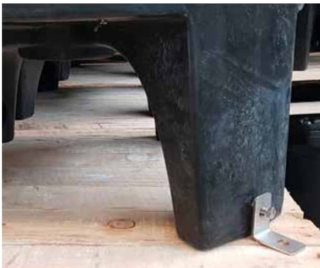
Figure 4 - Bolting the feet.
