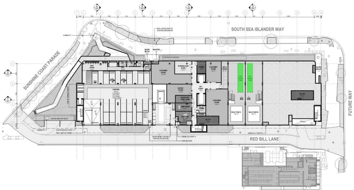
Figure 1: Location of the diesel storage tanks highlighted in green (Source: SC2-ARC-ARC-DRG-A-0100-3000, Rev 21)
