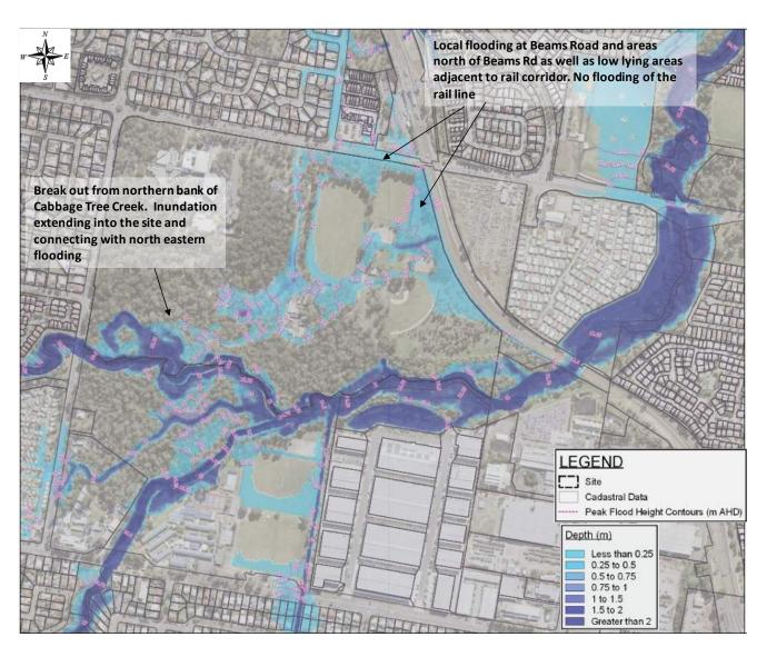
Figure 15 5% AEP flood inundation - existing conditions
