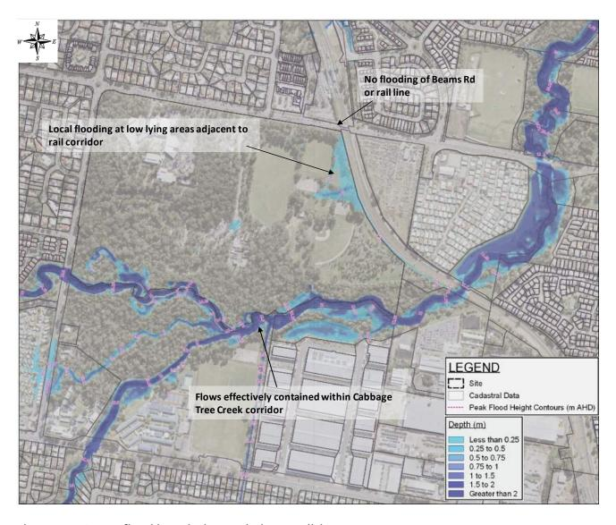
Figure 14 39% AEP flood inundation - existing conditions
