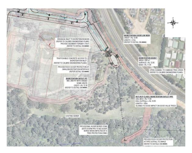
Figure 6 Bioretention basin B1 general arrangement
