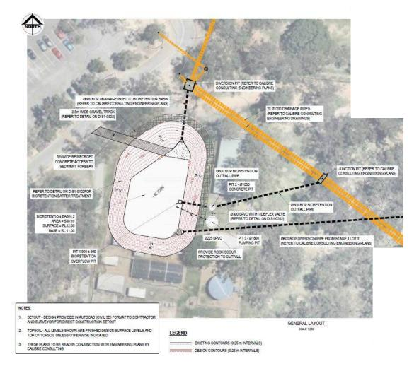
Figure 7 Bioretention basin B2 general arrangement
