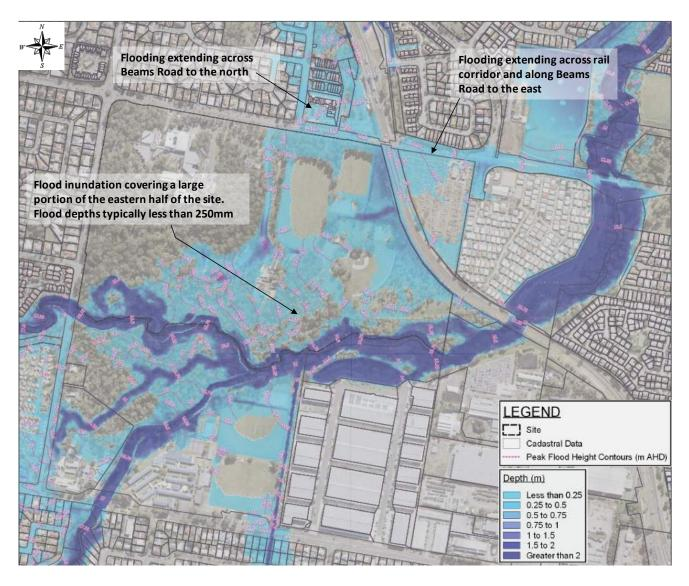
Figure 16 1% AEP flood inundation - existing conditions
