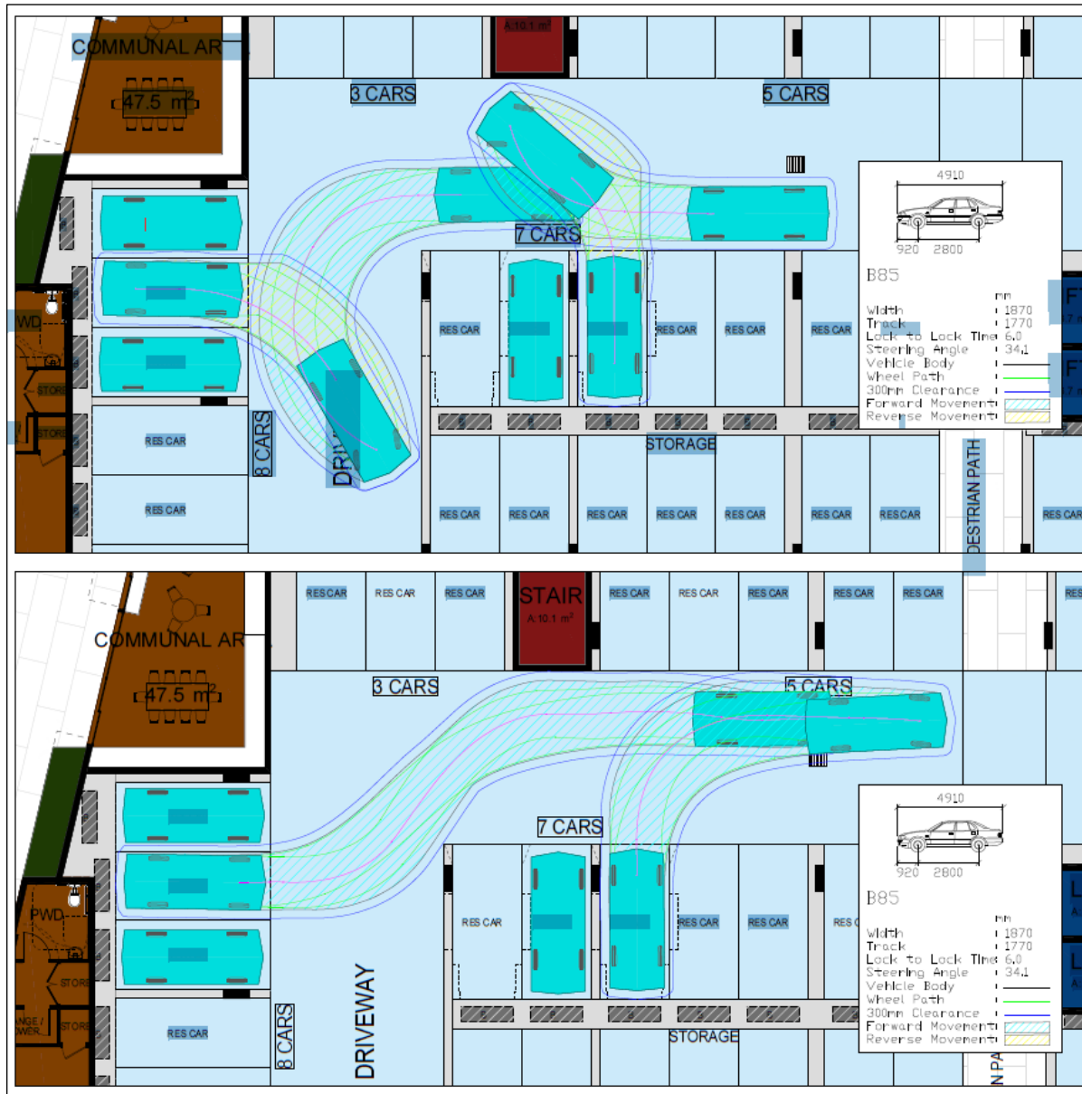
FIGURE 5.2 – SWEEP PATH OF 85 TH PERCENTILE VEHICLES
