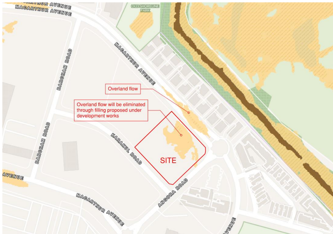
Figure 2: Overland Flow (BCC's GIS Flood Mapping, 2024)
