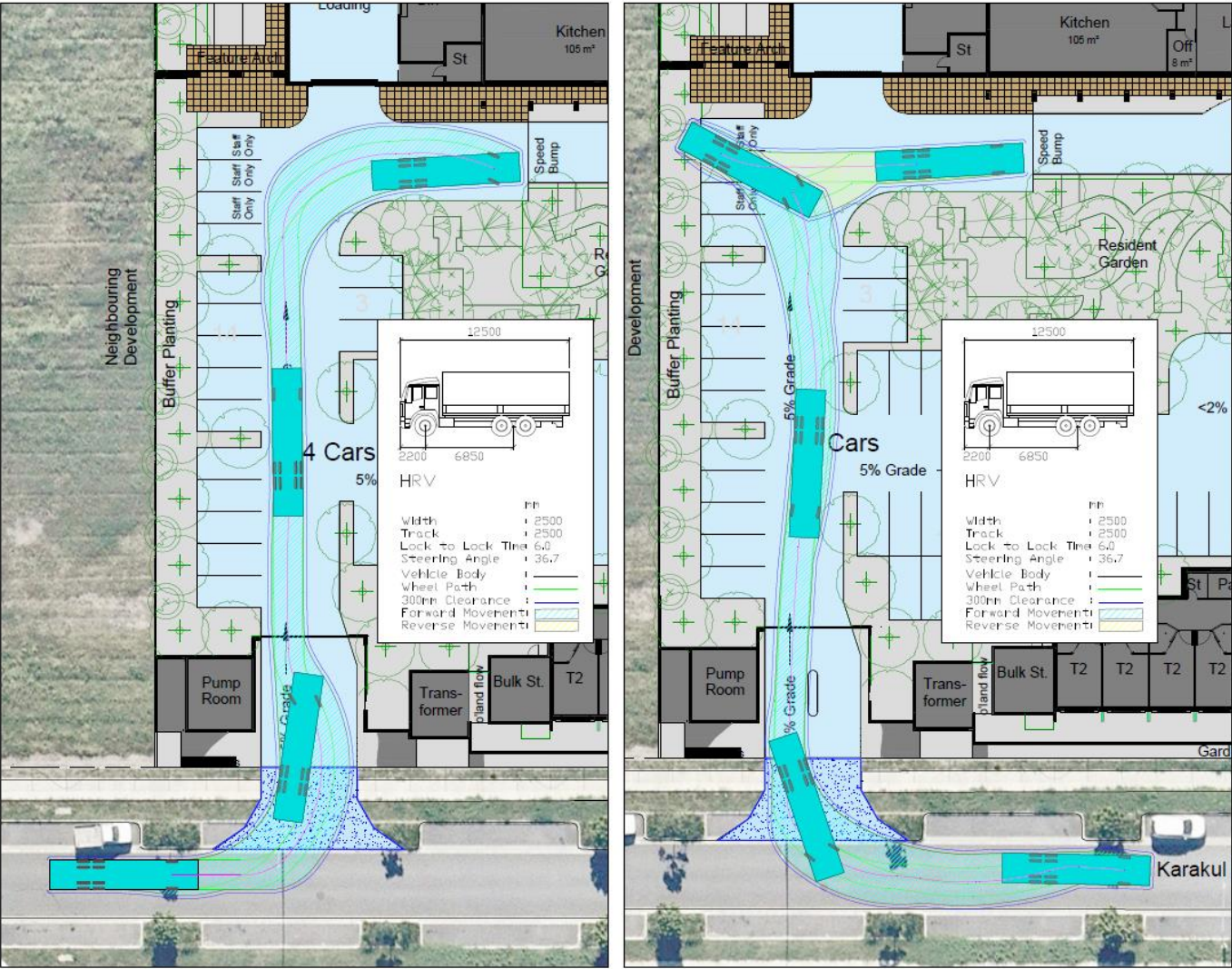
FIGURE 6.3 – SWEEP PATHS FOR A HEAVY RIGID VEHICLE (HRV)
