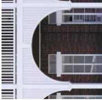
PT 3 WHITE PAINT TO ALL TIMBER WORK NEW PAINT TO MATCH EXISTING
