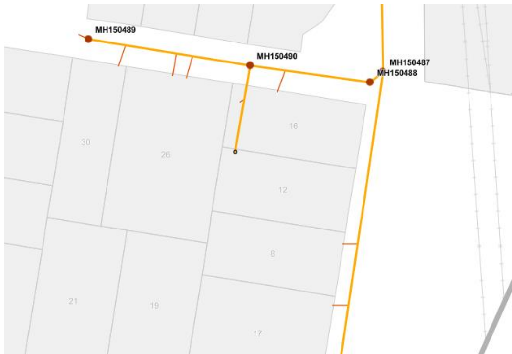
Figure 7 - BCC GIS Mapping – Sewer Infrastructure
