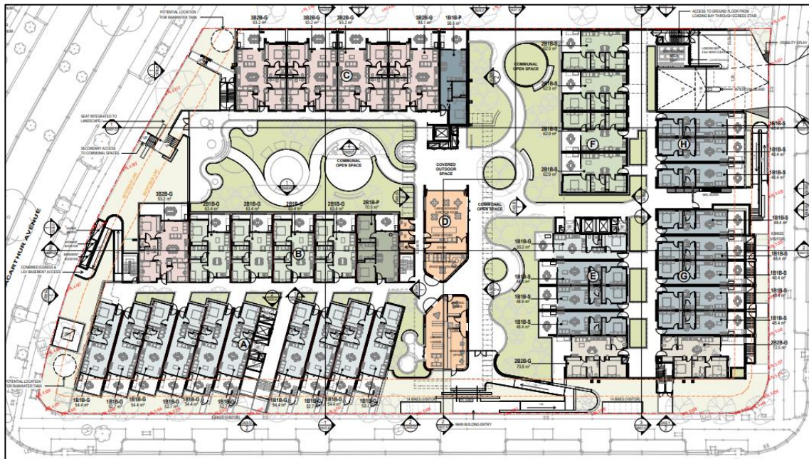
Figure 28: Brisbane Housing Company proposal (adjoining subject site to the west) – Ground floor plan showing 2 separate complexes with connected built form of multiple buildings (Source: Hayball proposal plans)
