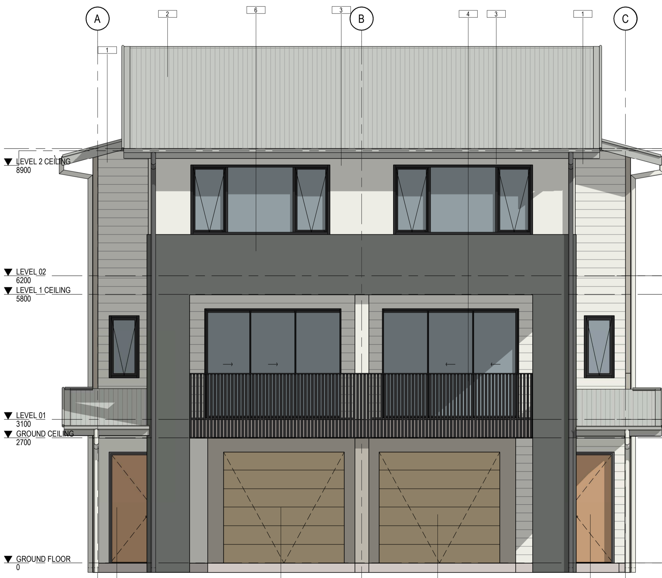
2 SOUTH ELEVATION COLOURED 1:50
