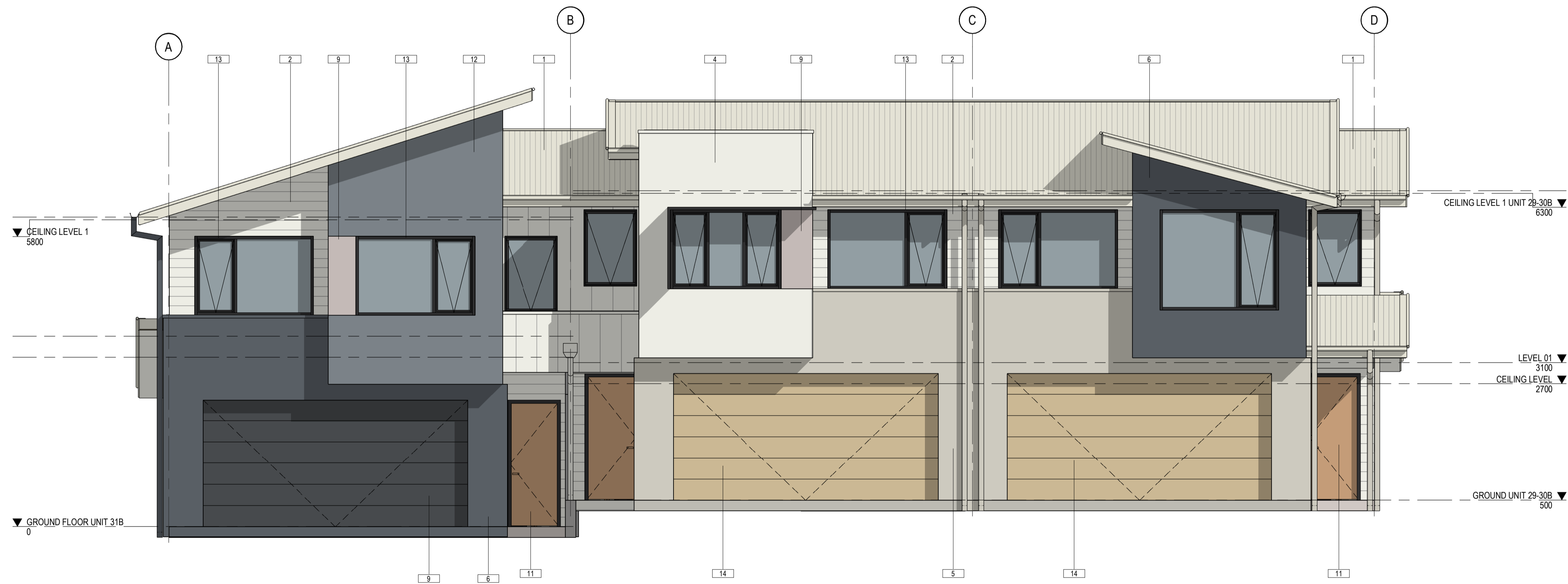
1 NORTH ELEVATION COLOURED A1-3-01/ 1:50
