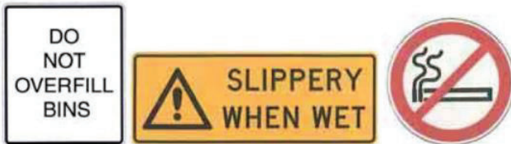
Figure I3.1: Example safety signs
