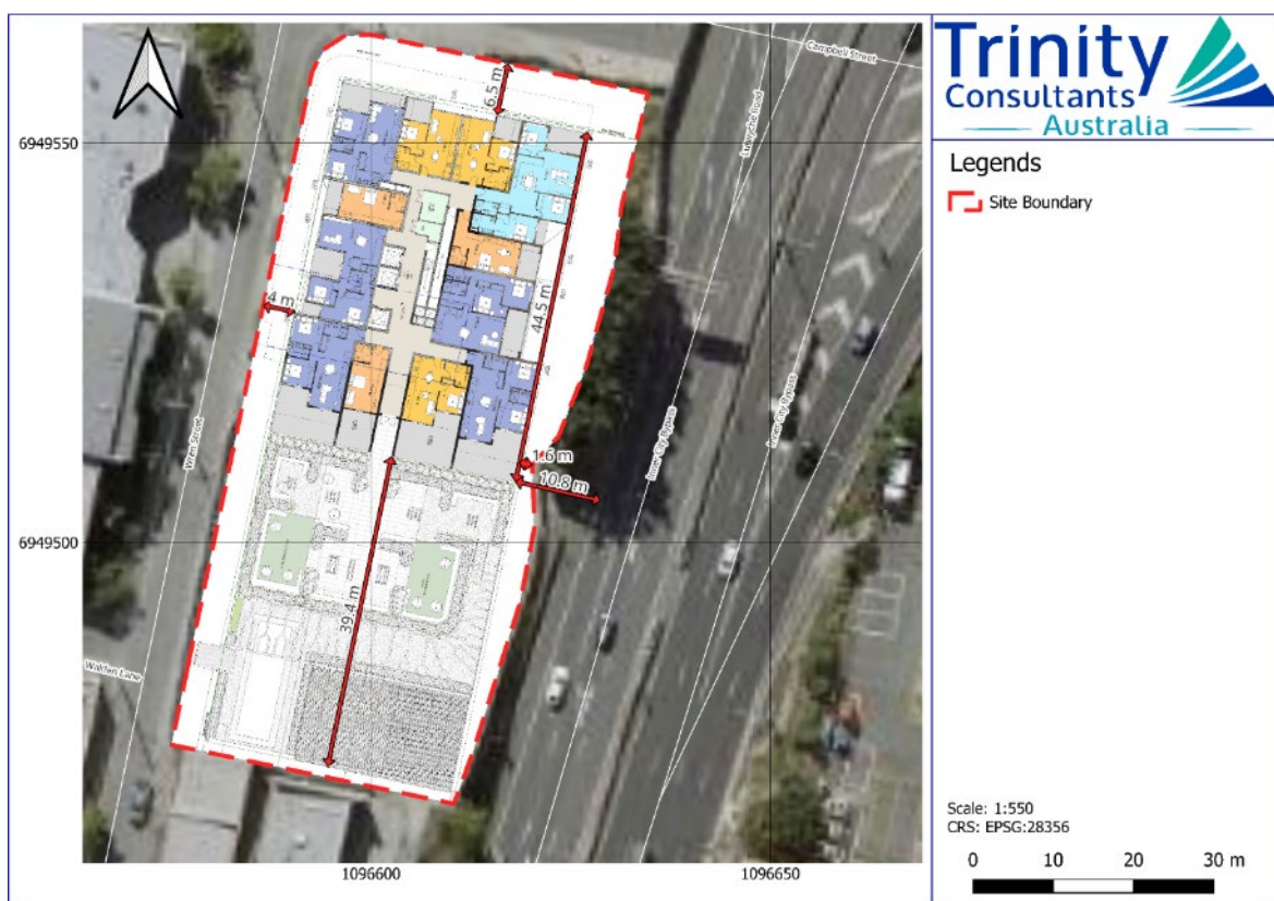
Figure 10.15: Separation Distances at Level 12
