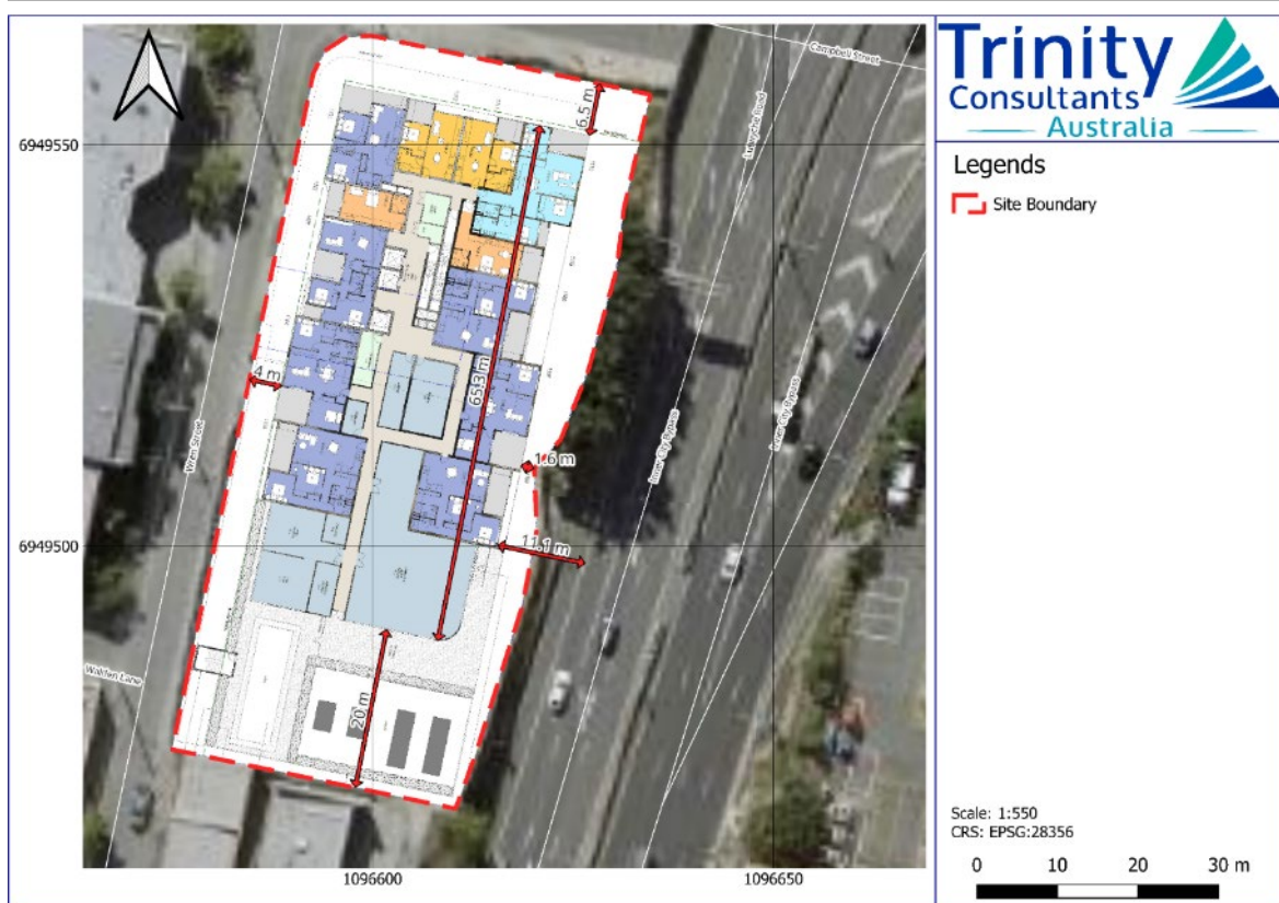
Figure 10.14: Separation Distances at Level 11
