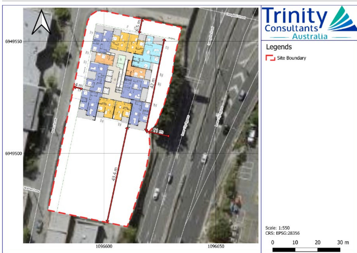
Figure 10.16: Separation Distances at Level 13 to Level 29
