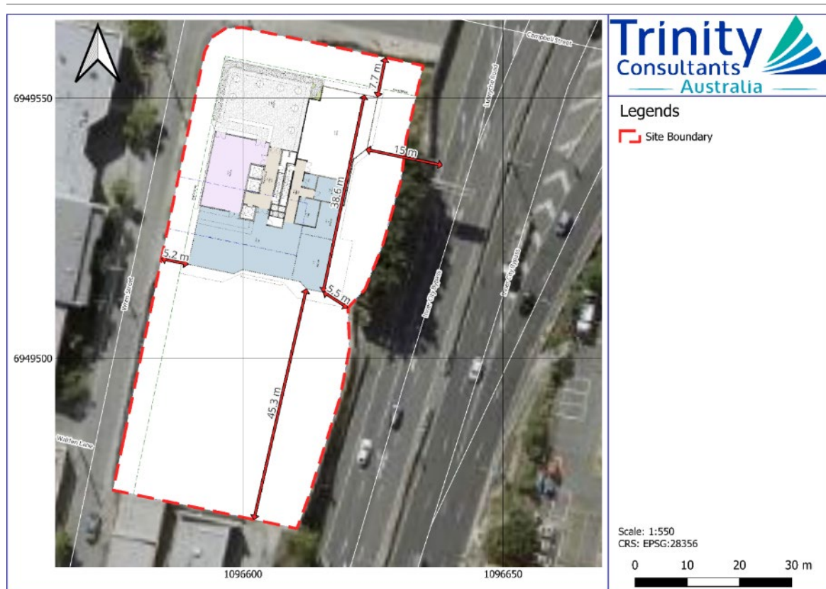
Figure 10.17: Separation Distances at Rooftop Level
