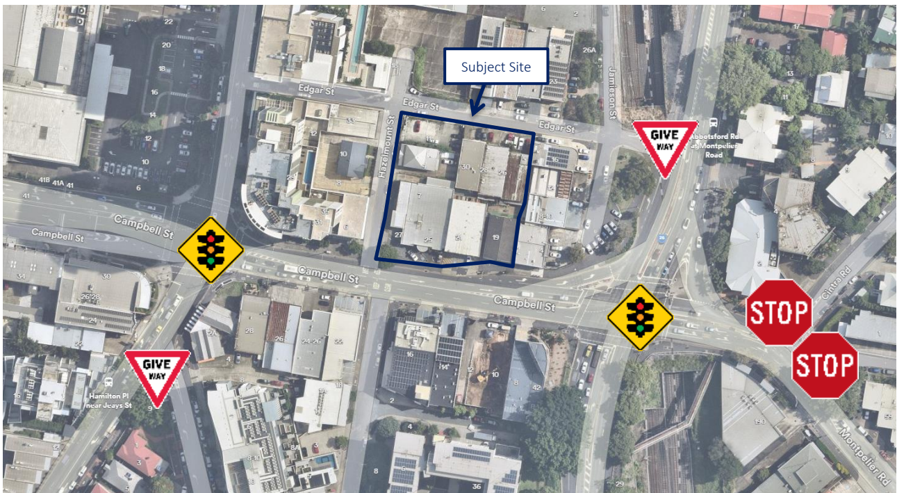
Figure 3.3: Existing Intersection Treatments
